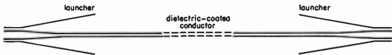
Fig. 17—Surface-wave transmission line with launchers at each end. These form transitions to coaxial line. Courtesy of Electronics
