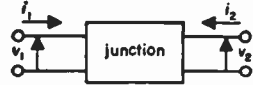
Fig. 13—Sign convention for defining the impedance and admittance of a 2-port junction.
