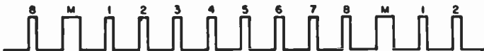
Fig. 10—Time-multiplex train of subcarrier pulses for 8 channels and marker pulse M for synchronization of receiver with transmitter.
