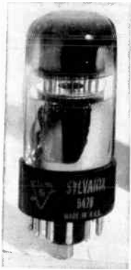
Fig. 8·34 A 6476 cold-cathode decade counter tube. (Sylvania Electric Products, Inc.)
