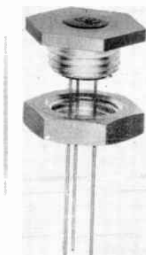
Fig. 3·3 A power transistor housed in a metallic container. The unit shown will provide a maximum power output of 6 watts when operated class A. (Minneapolis-Honeywell Regulator Co.)
