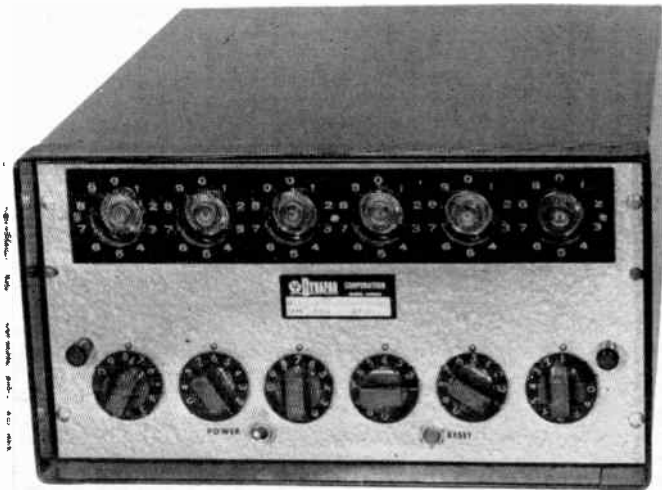
Fig. 8-33 A transistorized preset counter. This instrument contains two identical sets of counting circuits to enable it to perform a dual function. One counting circuit is shown in Fig. 8-37. (Dynapar Corp.)
