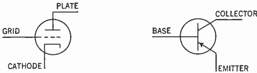
Fig. 3-28 Comparable elements in tubes and transistors: grid and base, cathode and emitter, and plate and collector.
