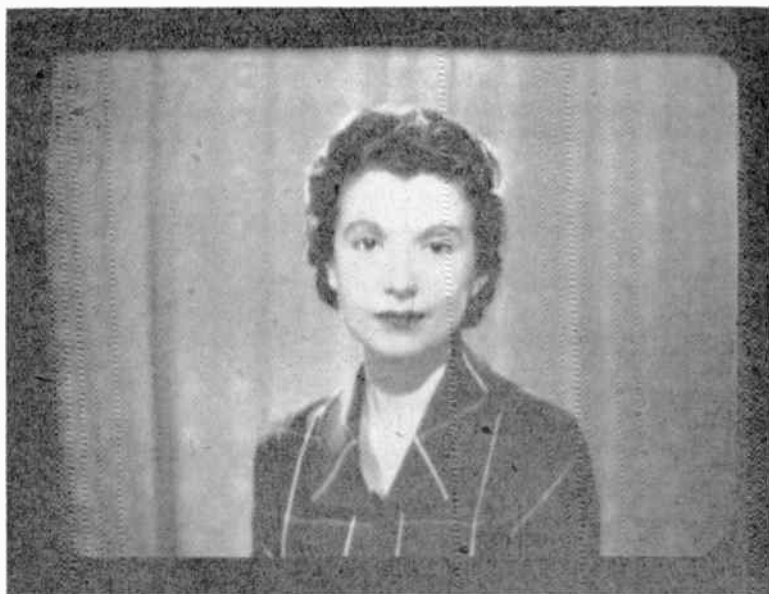
Fig. 36—Reproduced image from an image iconoscope with photo-electron stabilisation
