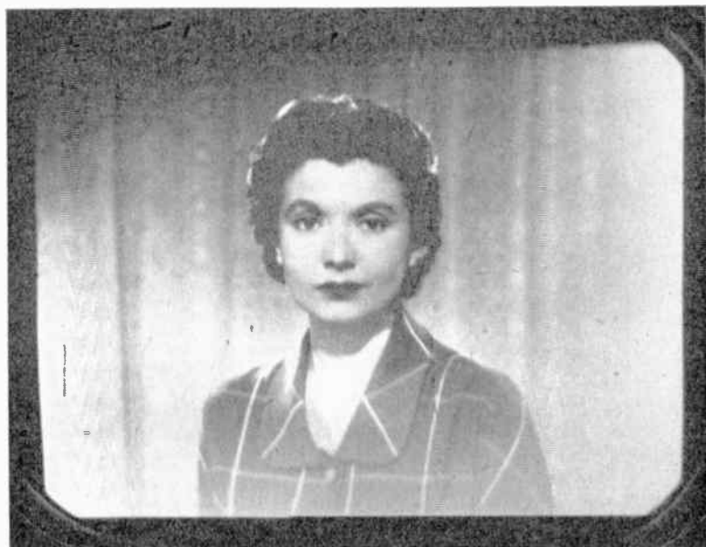
Fig. 37—Reproduced image from an image iconoscope without photo-electron stabilisation
