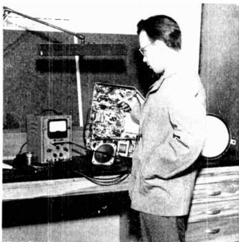
Figure 79. Proper method for taking high voltage measurements.
