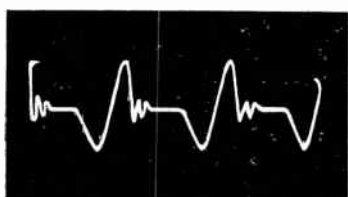
Fig. 60 12AU7 (V21) Horizontal Oscillator Section Plate (Pin 1) 40 volts P/P (Horizontal)
