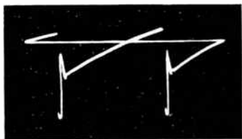
Fig. 63 12AU7 (V15) Vertical Oscillator Section Plate (Pin 1) 135 volts P/P (Vertical)
