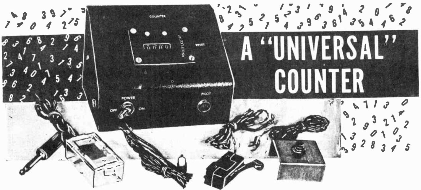
Fig. 1. Over-all view of the home-built counter with its associated accessories (from left to right): selenium photocell, mercury switch, the "Microswitch", and push-button switch.
