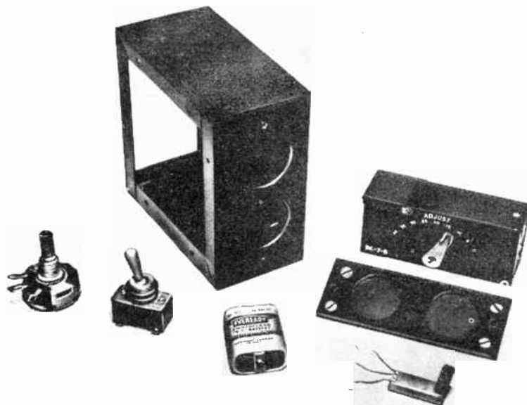
Photo of all parts used in the relay. The transistor, used in other experiments, is cemented to a small plastic block which supports its fragile leads.
