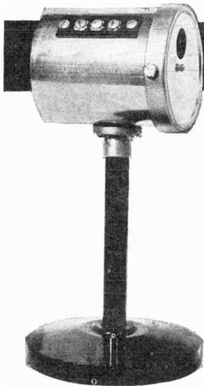
Fig. 1. Over-all view of author's unit. A discarded exposure meter cell was used.
