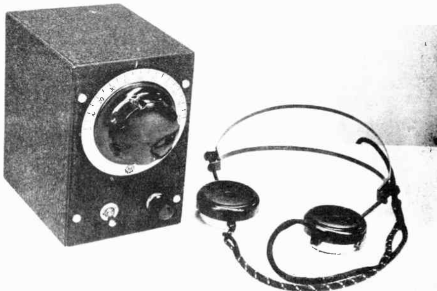
Over-all view of the experimental transistor receiver showing accessory headphones.
