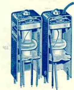
Inside view of I.F. transformers. The output type usually has four leads at the bottom. The input and interstage types have the grid lead coming out of the top.
