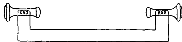
FIG. 9-4 ELEMENTARY TELEPHONE CIRCUIT
