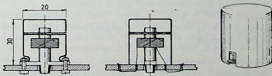
Fig. 94. Construction of the I.F. transformer.
