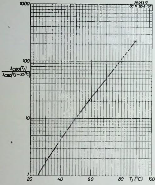
Fig. 14. Collector cut-off current versus junction temperature in common base connection.
