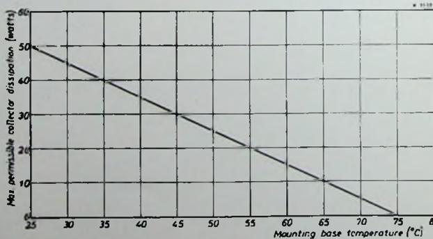
Fig. 2. The permissible collector dissipation is determined by the mounting base temperature. The mounting base temperature depends on the cooling capacity of the chassis or some other heat dissipating medium to which the transistor is attached.
