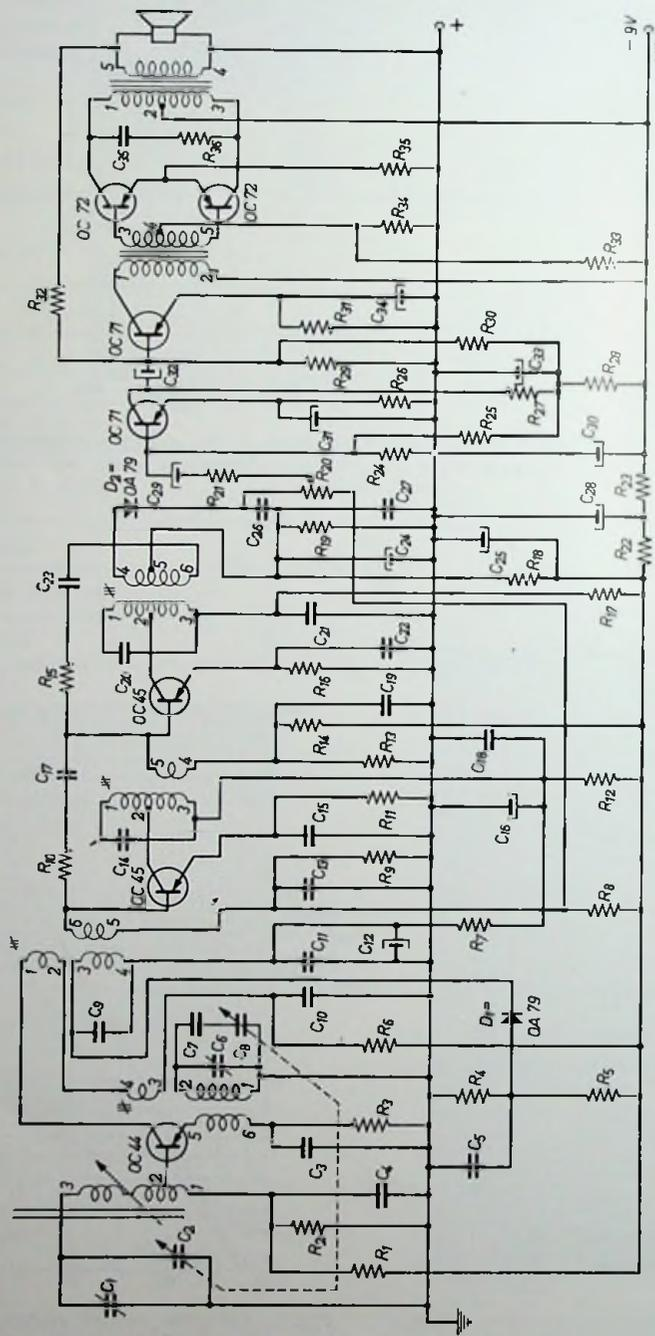
Fig. 8. Circuit diagram of an experimental all-transistor superhetro receiver.
