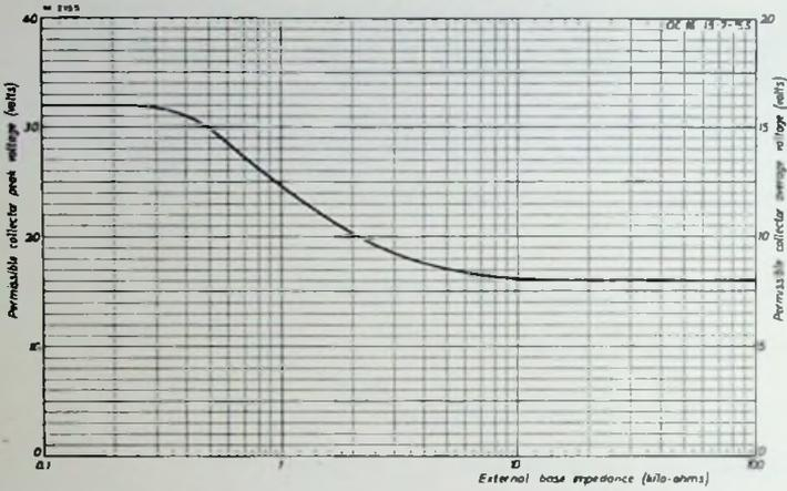
Fig. 11. The maximum permissible average and peak value of the collector-to-emitter voltage as a function of the external impedance between base and emitter. Provisions must be made to ensure thermal stability.
