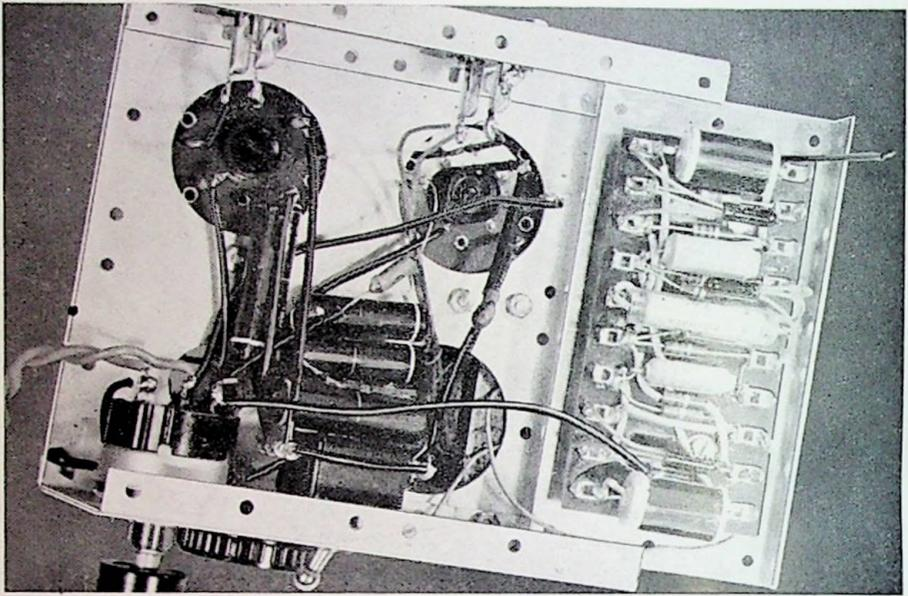
Nevertheless, experience has shown that the circuit provides sufficient amplification to permit a certain amount of negative feedback ( $R_f$ ) to be employed, which improves the quality of reproduction.
