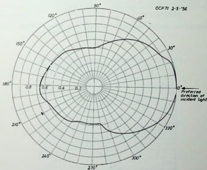
Fig. 4. Relation between the sensitivity and direction of incident light.
