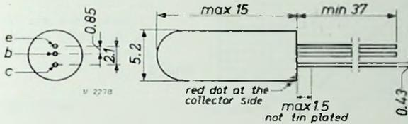
Fig. 1. Dimensional outline in mm and electrode connections.
