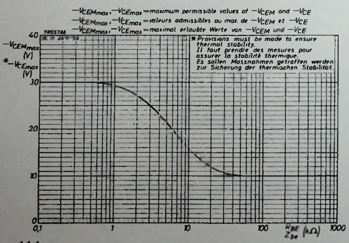
Fig. 16. The maximum permissible average and peak value of the collector-to-emitter voltage as a function of the external impedance between base and emitter.
