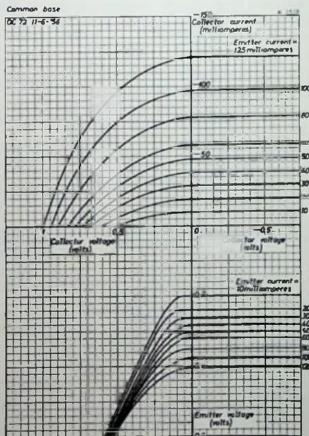
Fig. 12. Typical low-voltage characteristics of the OC 72 in common base connection at constant junction temperature.
