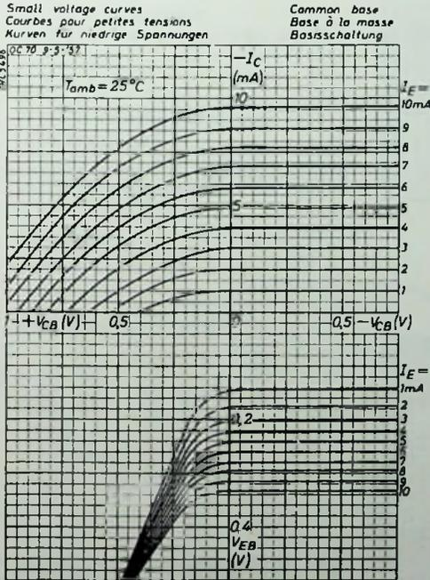
Fig. 12. Typical low-voltage characteristics in common base connection at an ambient temperature of 25 °C.
