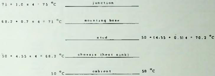
Fig. 8. Temperature scale for  $W_c = 4 \text{ W}$ ,  $t_{amb} = 50 \text{ }^\circ\text{C}$ .
