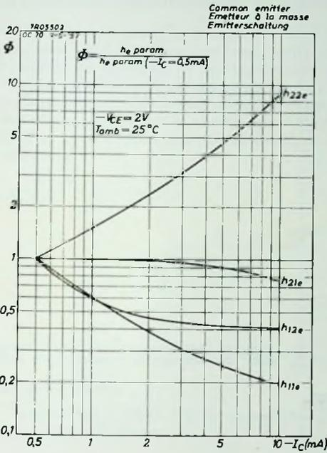
Fig. 10. h-parameters versus collector current in common emitter connection at an ambient temperature of 25 °C.
