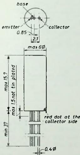
Fig. 1. Dimensional outline in mm and electrode connections.
