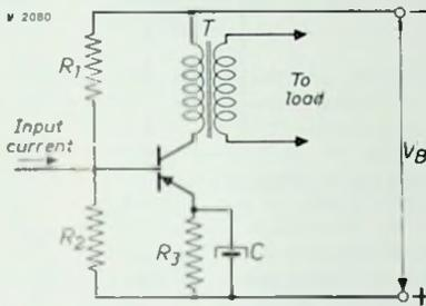
FIG. 6. Class A amplifying stage with a transistor OC 72.
