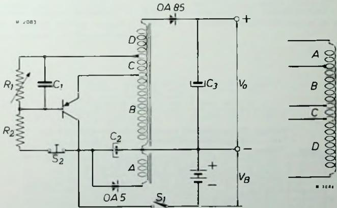
Fig. 6. D.C. converter with a transistor OC 76 without cooling fin. By means of the switches  $S_1$  and  $S_2$  which are mechanically coupled so that  $S_2$  is opened after  $S_1$  has been closed, the oscillation is initiated.
