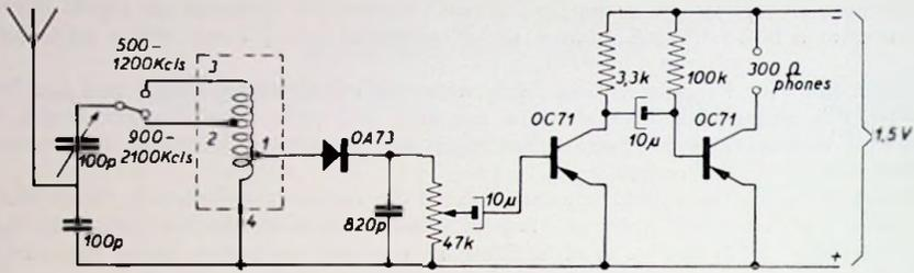
Fig. 71. The tuning coil is wound on a former with flanges at distances of 2 mm and an outer diameter of 20 mm and a breadth of 12 mm at the bottom. A powdered iron core should be inserted. The total number of turns is 360. Litz wire  $16 \times 0.04$  mm. Start winding at connection no. 4; make tap no. 1 at 24 turns, no. 2 at 220 turns.
