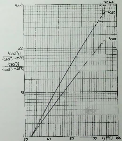
Fig. 7. Collector cut-off current in common base ( $I_{CBO}$ ) and in common emitter ( $I_{CEO}$ ) as a function of the junction temperature.
