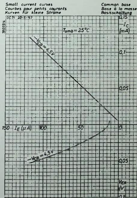
Fig. 13. Typical low-current characteristics in common base connection at an ambient temperature of  $25^\circ \text{ C}$ .
