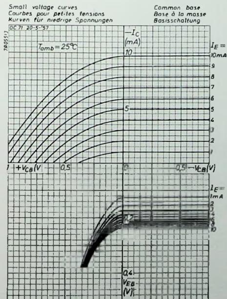
Fig. 12. Typical low-voltage characteristics in common base connection at an ambient temperature of  $25^\circ \text{ C}$ .
