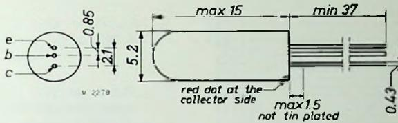
Fig. 1. Dimensional outline in mm and electrode connections.
