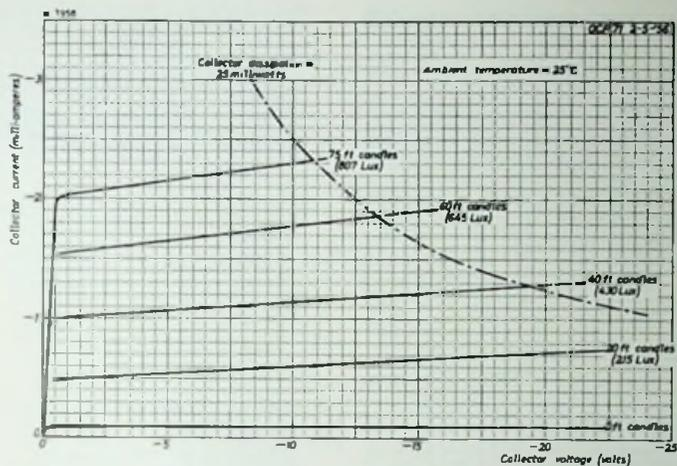
Fig. 3. Typical characteristics of the OCP 71.
