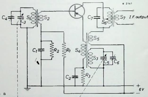
Fig. 5. Self-exciting convertor with a transistor OC 44.
