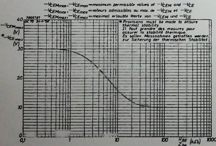
Fig. 16. The maximum permissible average and peak value of the collector-to-emitter voltage as a function of the external impedance between base and emitter.
