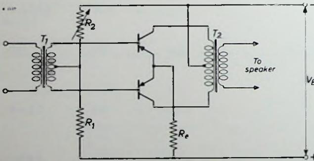
Fig. 4. Output stage with a matched pair of transistors 2-OC 16 in a class B amplifier
