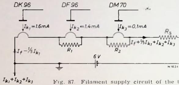
Fig. 87. Filament supply circuit of the tubes.
