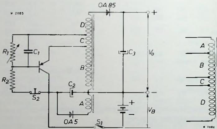
Fig. 8. D.C. converter with a single transistor OC 72 without cooling fin. By means of the switches \$S\_1\$ and \$S\_2\$ which are mechanically coupled so that \$S\_2\$ is opened after \$S\_1\$ has been closed, the oscillation is initiated.
