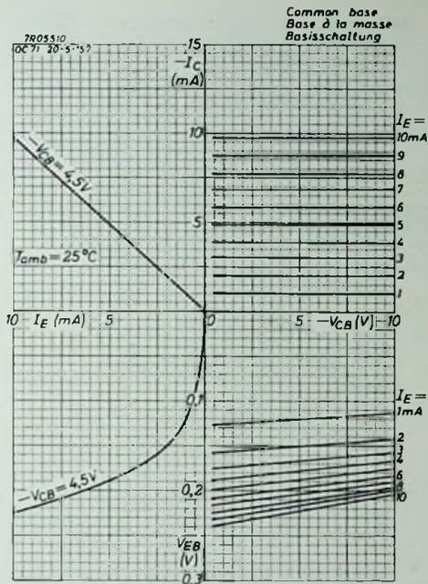
Fig. 11. Typical characteristics in common base connection at an ambient temperature of  $25^\circ \text{ C}$ .
