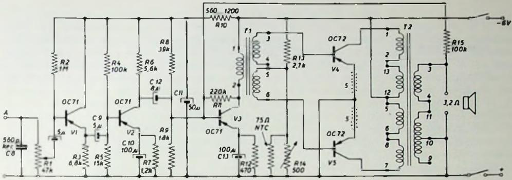
Fig. 76. Low-frequency part of 5-transistor receiver, to be combined with the band-filter unit of Fig. 72.
