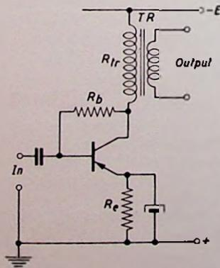
Accordingly, the efficiency of the system is  $\frac{W_o}{W_b} \cdot 100\% = 50\%$ .
