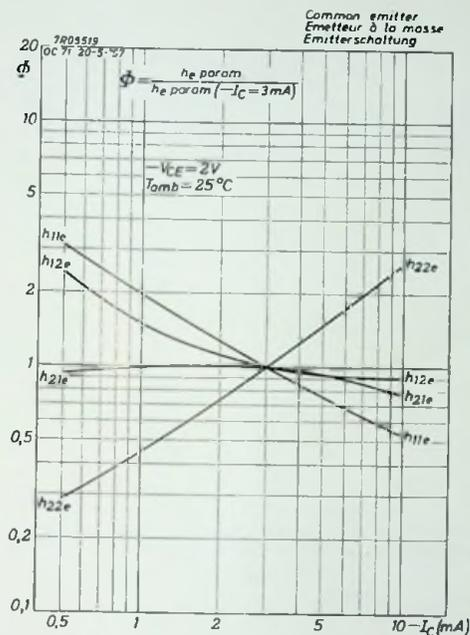
Fig. 10.  $h$ -parameters versus collector current in common emitter connection at an ambient temperature of  $25^\circ \text{ C}$ .
