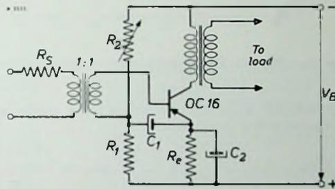
Fig. 5. Class A amplifying stage with a transistor OC16
