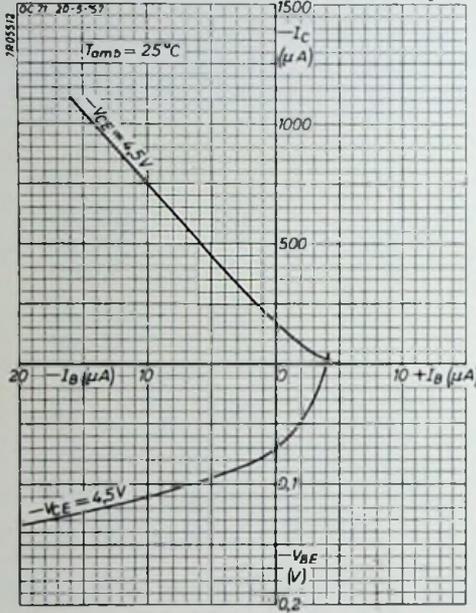
Fig. 6. Typical low-current characteristics in common emitter connection at an ambient temperature of 25 °C.
