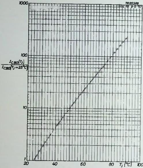
FIG. 14. Collector cut-off current versus junction temperature in common base connection
