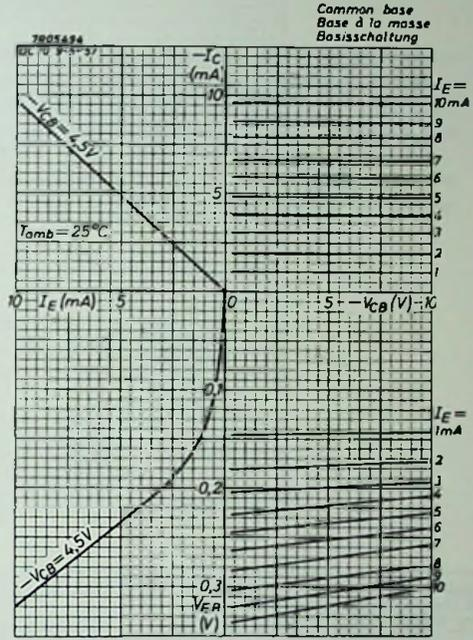
Fig. 11. Typical characteristics in common base connection at an ambient temperature of 25 °C.
