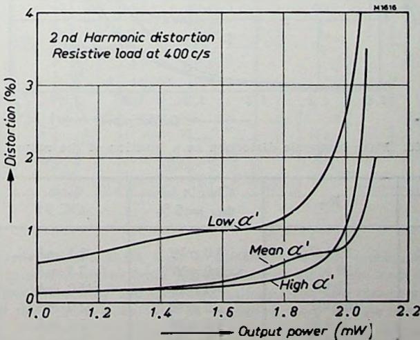
Fig. 61. Second harmonic distortion as a function of the output power.
