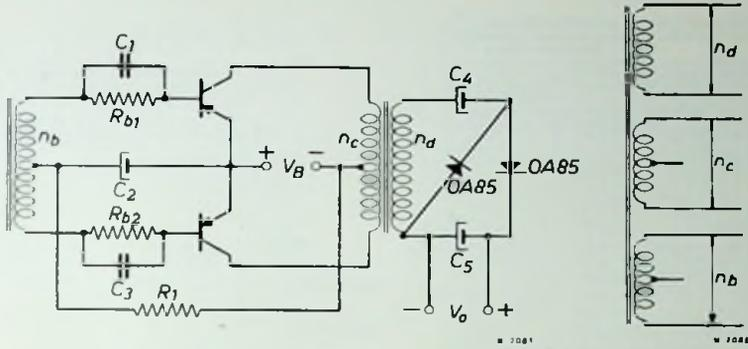
Fig. 5. Push-pull D.C. converter with two transistors OC 76 without cooling fin.
