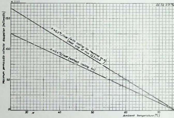
Fig. 3. Maximum permissible collector dissipation as a function of the ambient temperature.
