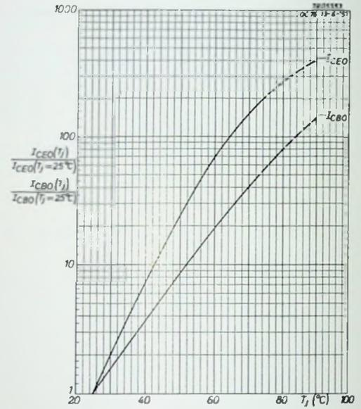
Fig. 8. Collector cut-off current in common base ( $-I_{CB0}$ ) and in common emitter ( $-I_{CE0}$ ) as a function of the junction temperature.
