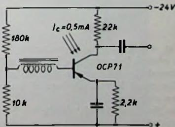
Fig. 42. Stabilised circuit for modulated light.
