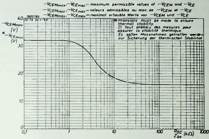
Fig 13. The maximum permissible average and peak value of the collector-to-emitter voltage as a function of the external impedance between base and emitter. Provisions must be made to ensure thermal stability.
