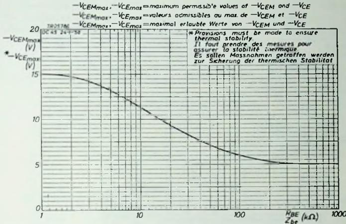
Fig. 6. The maximum permissible average and peak value of the collector-to-emitter voltage as a function of the resistance between base and emitter. Provisions must be made to ensure thermal stability.
