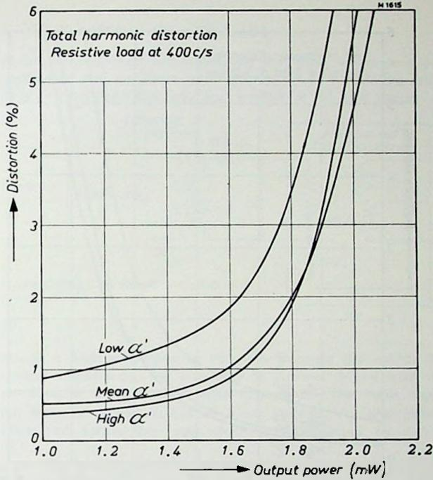
Fig. 60. Total harmonic distortion as a function of the output power.
