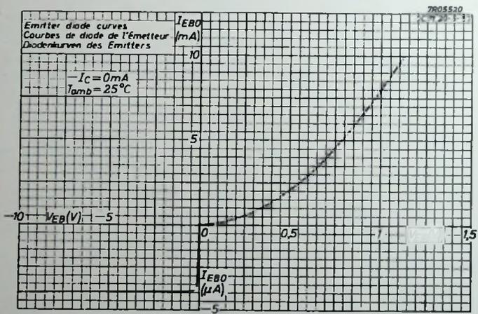
Fig. 15. Typical emitter diode characteristic at an ambient temperature of 25 °C.
