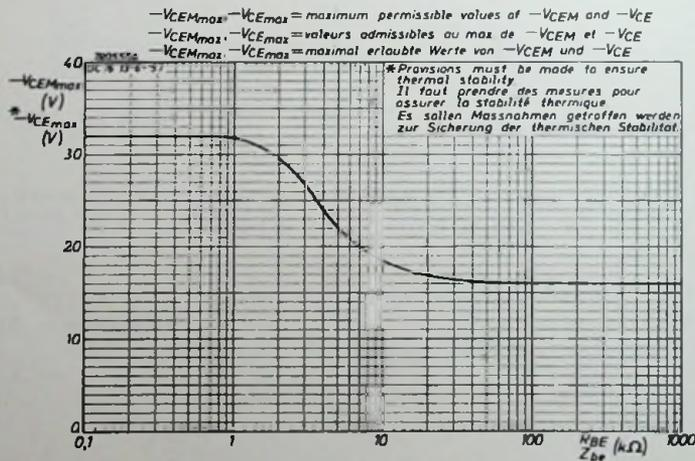
Fig. 9. The maximum permissible average and peak value of the collector-to-emitter voltage as a function of the external impedance between base and emitter.
