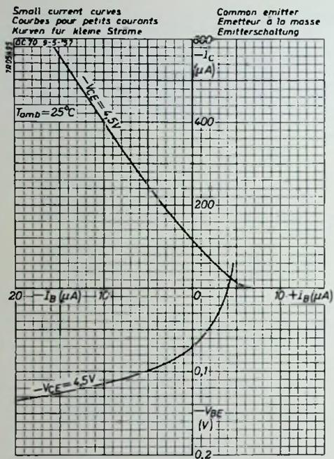
Fig. 6. Typical low-current characteristics in common emitter connection at an ambient temperature of 25 °C.
