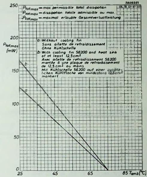
Fig. 3. Maximum collector dissipation as a function of the ambient temperature.
