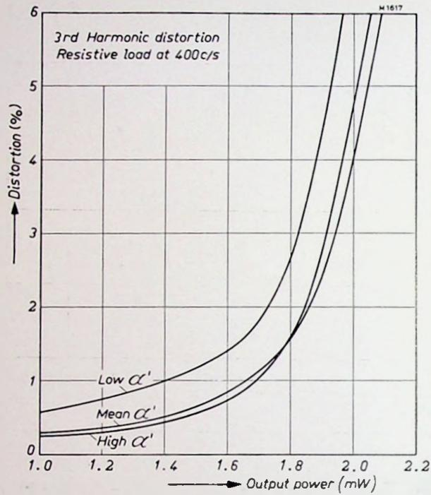
Fig. 62. Third harmonic distortion as a function of the output power.
