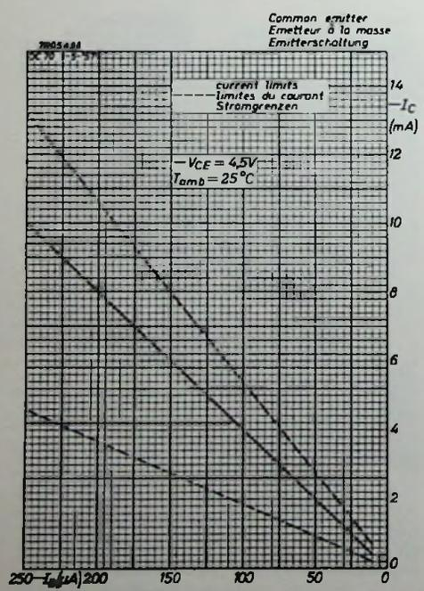
Fig. 8. Current amplification characteristics in common emitter connection at an ambient temperature of 25 °C.
