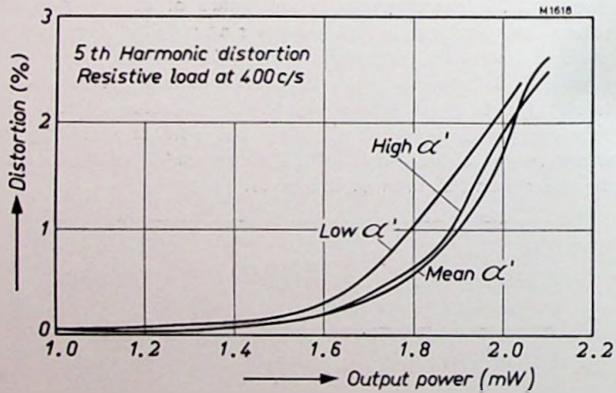
Fig. 63. Fifth harmonic distortion as a function of the output power.
