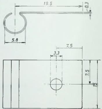
Fig. 2. Dimensions of the cooling fin, which is separately available under type number 56200
