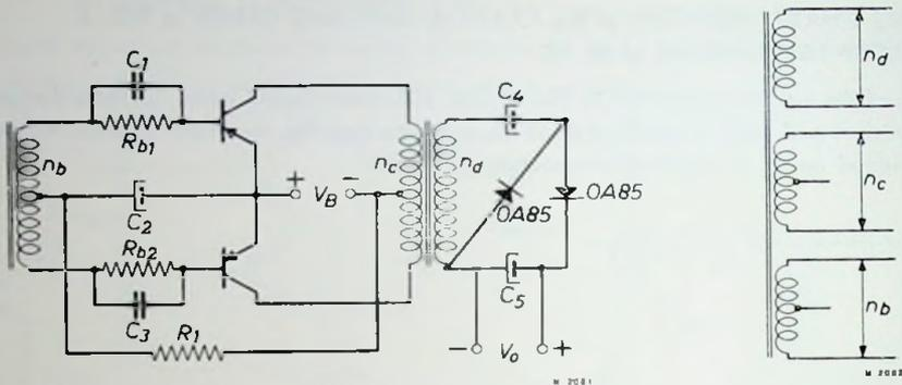
Fig. 7. Push-pull D.C. converter with two transistors OC 72 without cooling fin.
