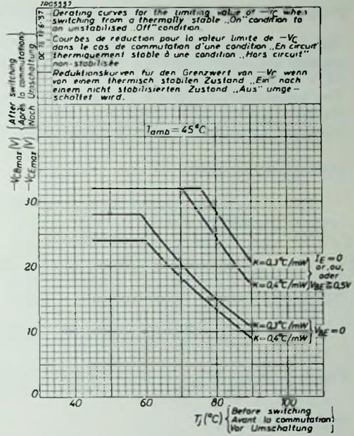
Fig. 11. Collector voltage derating curves at an ambient temperature of  $45^\circ\text{C}$ .
