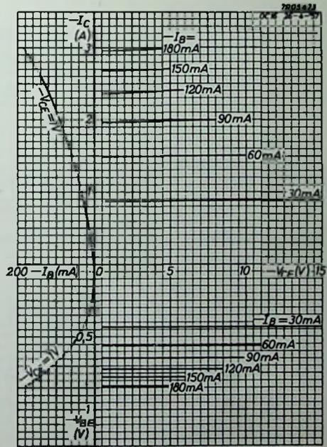
Fig. 10. Typical characteristics of the OC 16 in common emitter connection at a junction temperature of 45 °C.
