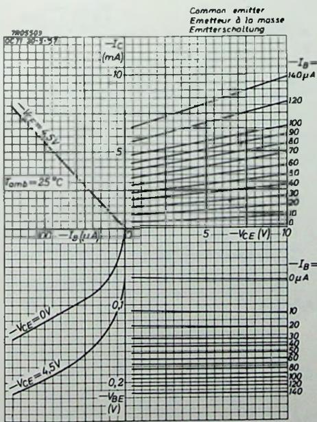
Fig. 4. Typical characteristics in common emitter connection at an ambient temperature of 25 °C.
