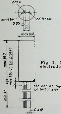
Fig. 1. Dimensional outline in mm and electrode connections of the transistor OC 76
