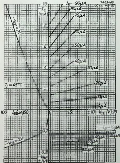
Fig. 6. Typical characteristics of the OC 44 in common emitter connection at a junction temperature of 45 °C.
