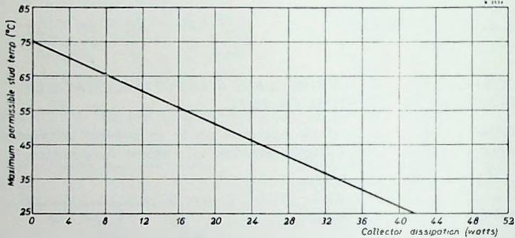
Fig. 6. Permissible stud temperature versus collector dissipation
