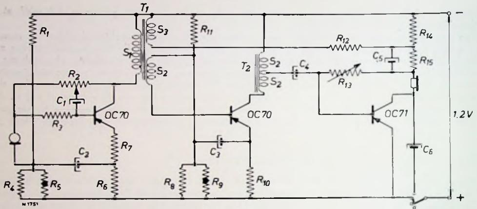
Fig. 56. Circuit of a transformer-coupled hearing aid with three transistors.
