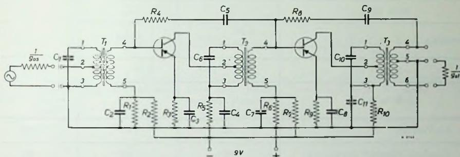
Fig. 4. Basic circuit of a two-stage I.F. amplifier. The design of this circuit provides stable operation and interchangeability of the transistors.
