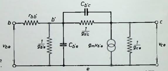
Fig. 3. Hybrid  $\pi$  equivalent circuit. The internal base connection is indicated by  $b'$ .
