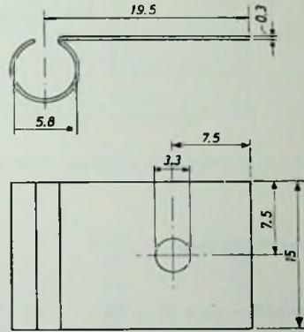
Fig. 2. Dimensions of the cooling fin, which is separately available under type number 56200.
