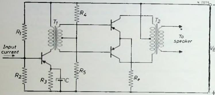
Fig. 5. Output stage with a matched pair of transistors 3-OC 72 in a class B amplifier and a transistor OC 71 in the driver stage.
