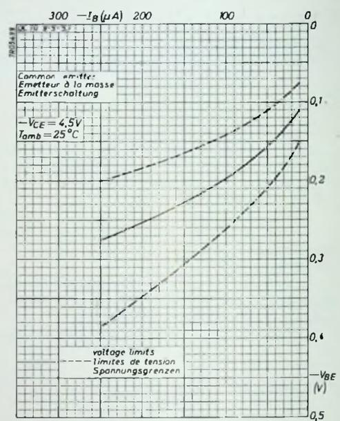
Fig. 7. Input characteristics in common emitter connection at an ambient temperature of 25 °C.
