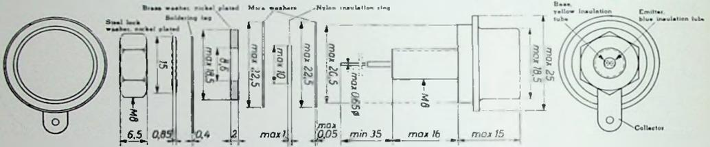
Fig. 1. Dimensional outline (in mm) and electrode connections. The collector is connected to the case; mica washers to insulate the case from the chassis are provided.
