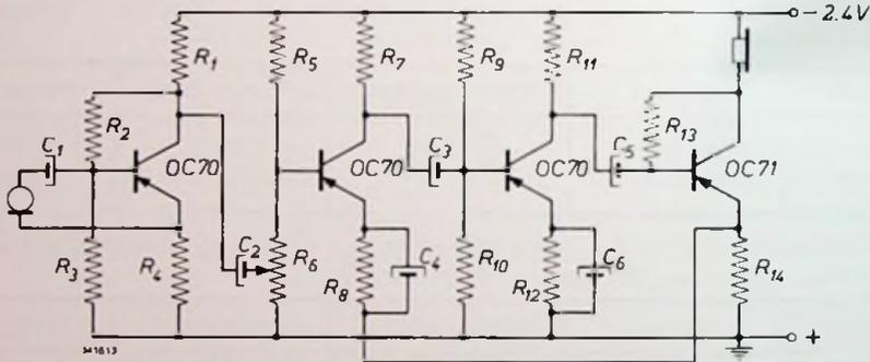
Fig. 58. Circuit of an RC-coupled hearing aid with four transistors.
