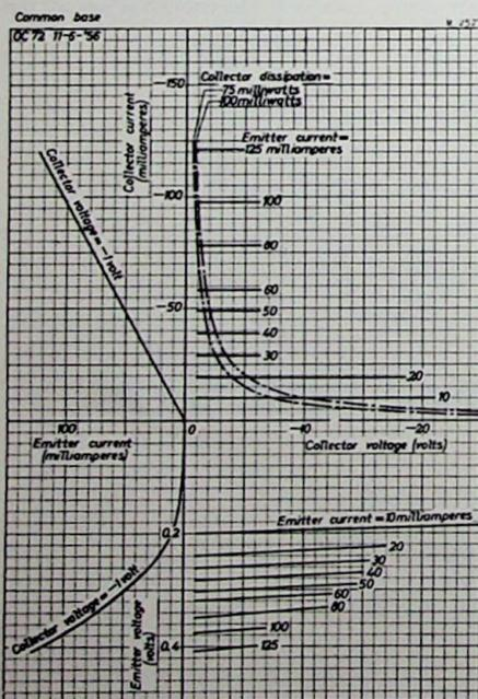
Fig. 11. Typical characteristics of the OC 72 in common base connection at constant junction temperature.
