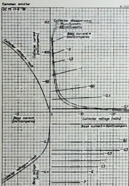
Fig. 9. Typical characteristics of the OC 72 in common emitter connection at constant junction temperature.
