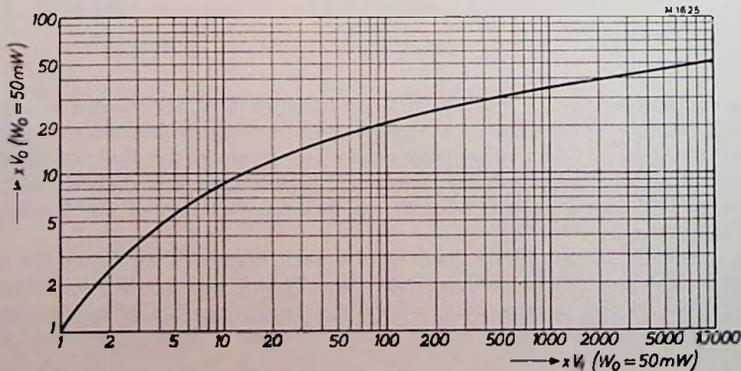
Fig. 88. A.G.C. curve of the receiver.
