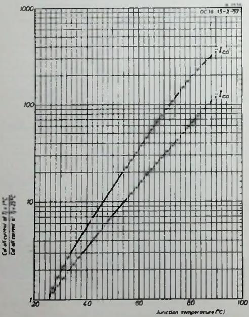
Fig. 12. Collector cut-off current in common base ( $I_{CB}$ ) and in common emitter ( $I_{CE}$ ) as a function of the junction temperature.
