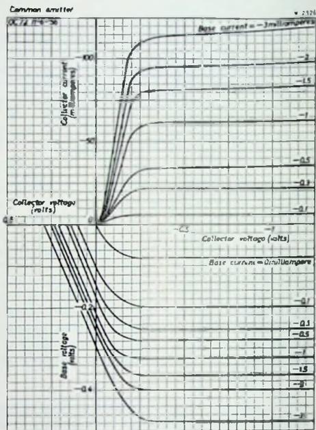
Fig. 10. Typical low-voltage characteristics of the OC 72 in common emitter connection at constant junction temperature.
