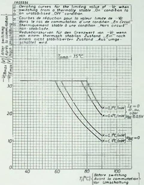
Fig. 10. Collector voltage derating curves at an ambient temperature of  $35^\circ\text{C}$ .
