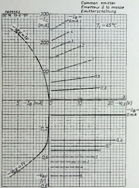
Fig. 7. Typical characteristics in common emitter connection at a junction temperature of  $45^\circ\text{C}$ .
