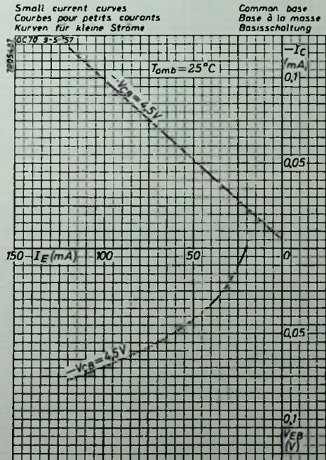
Fig. 13. Typical low-current characteristics in common base connection at an ambient temperature of 25 °C.
