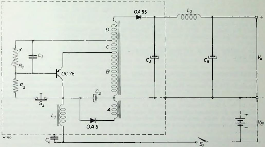
Fig. 97. Circuit of the d.c. convertor.
