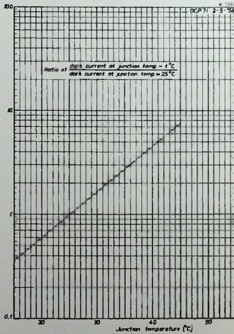
Fig. 7. Relation between dark current and junction temperature.
