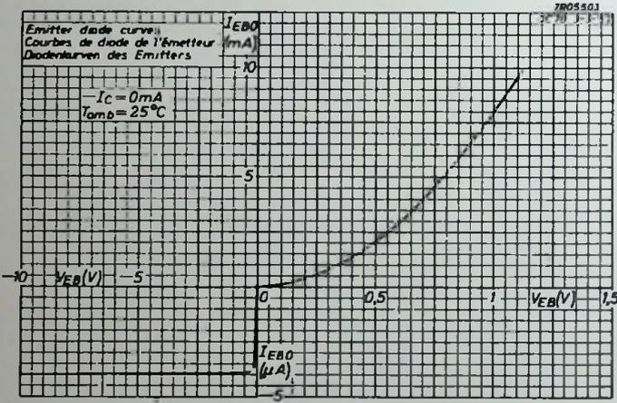
Fig. 15. Typical emitter diode characteristic at an ambient temperature of 25 °C.
