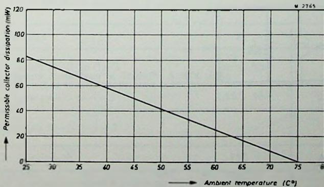
Fig. 2. Maximum continuous collector dissipation as a function of the ambient temperature.
