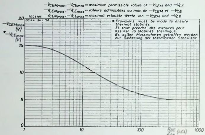
Fig. 8. The maximum permissible average and peak value of the collector-to-emitter voltage as a function of the impedance between base and emitter. Provisions must be made to ensure thermal stability.
