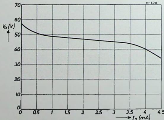
Fig. 99. Output voltage of the d.c. converter at varying load current.
