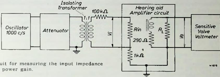
Fig. 64. Circuit for measuring the input impedance and power gain.
