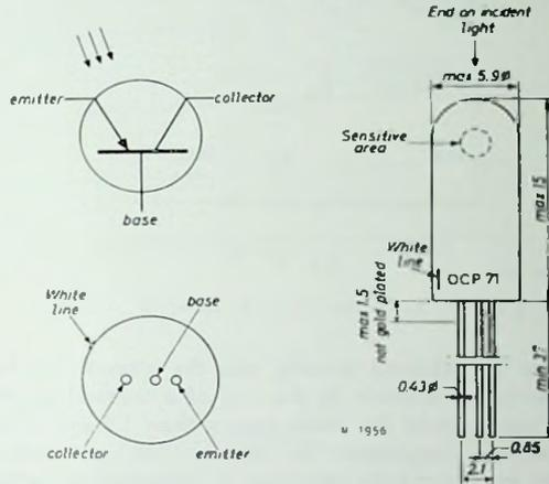
Fig. 1. Dimensional drawing (dimensions in mm) and electrode connections of the OCP 71. The preferred direction of incident light is perpendicular to the plane of the leads and is on the side of the bulb bearing the type number.
