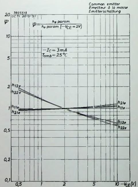
Fig. 9. h-parameters versus collector voltage in common emitter connection at an ambient temperature of 25 °C.
