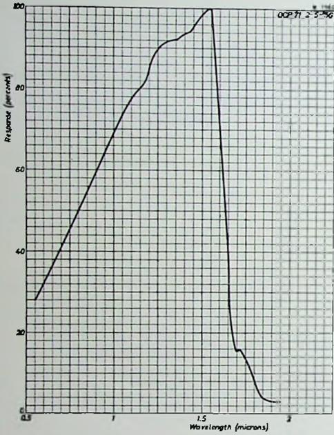
Fig. 5. Spectral response to constant energy spectrum.
