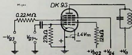
Fig. 84. Performance of the tube DK 96 as a function of the control-grid voltage ( $V_{g1}$ ), at a supply voltage of 45 V, in a circuit as indicated. The oscillator voltage ( $V_{g1}$ ) is 4  $V_{eff}$ .
