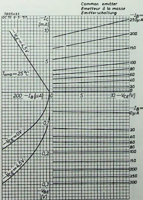
Fig. 4. Typical characteristics in common emitter connection at an ambient temperature of 25 °C.
