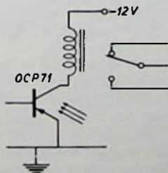
Fig. 41. Photo-transistor OCP 71 as photo-electric relay.
