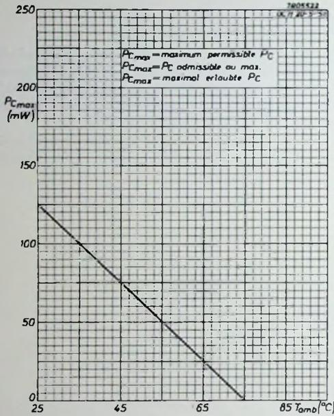
Fig. 2. Maximum collector dissipation as a function of the ambient temperature.
