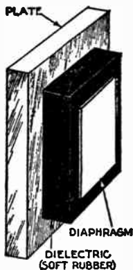
FIG. 12—Elements of an electrostatic speaker. It consists essentially of a form of condenser, hence the name as it is often called a condenser speaker.
