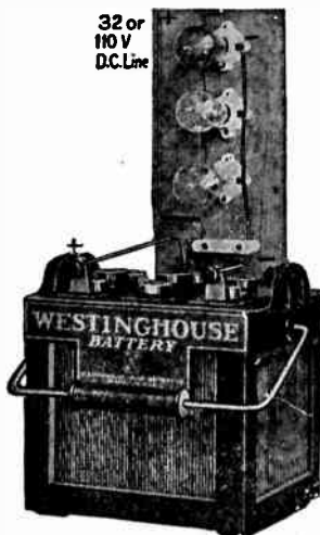
FIG. 18.—Set up showing connections for charging a 6 volt A battery from a 32 or 110 volt direct current line by means of a lamp bank. Adding lamps to the bank will increase the charge rate. Using lamps of larger wattage will also increase the charge rate.
