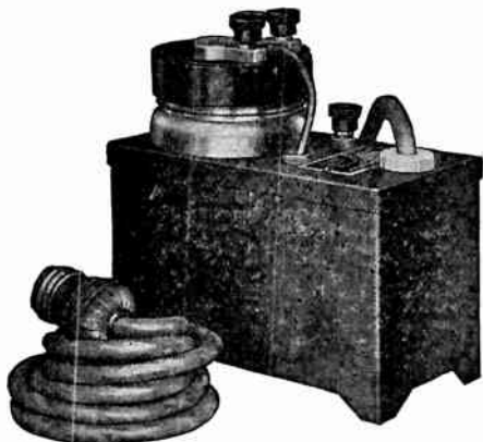
FIG. 13.—Globe Silite trickle charger. This charger uses the new metallic glass element, silite, adapted to storage batteries preferably not over 60 ampere hour capacity. This combination will meet the requirements up to six or eight tube sets which are not used on an average of more than four hours a day. Charges at .6 to .75 ampere rate and may be used with either 4 or 6 volt batteries.
