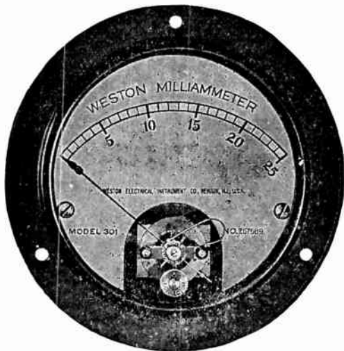
FIG. 3.—Weston plate or grid milli-ammeter for measuring the plate current of vacuum tubes. It will give a deflection for steady or pulsating direct current and will indicate the average value of a pulsating current. Superimposed upon the steady plate current is the current due to the modulation which is an alternating current and will cause the total plate current to be a pulsating current varying at the same frequency as the modulation current. The milli-ammeter will again indicate the average value of this current and if the tube be working as a point where it rectifies, this average value will not be the same as the value of the unmodulated steady plate current and therefore fluctuate with the modulation. For perfect reproduction, amplifying tubes should not rectify and no variation in the indication of the milli-ammeter should occur. In practice however, on account of the properties of vacuum tubes, some rectification will result, but by properly adjusting the grid bias, a minimum fluctuation in the plate current may be obtained consistent with good quality and volume.
