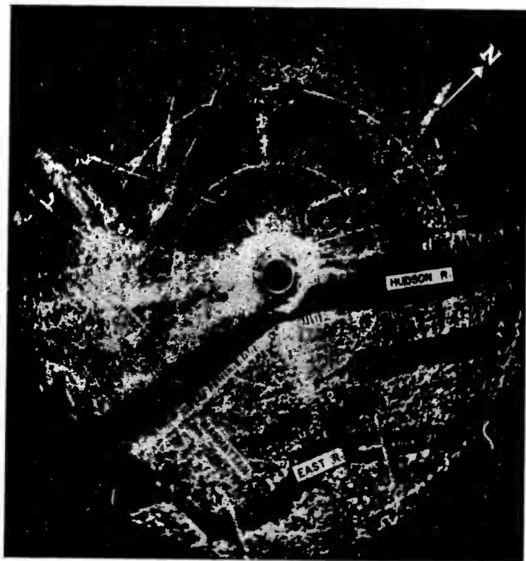
FIG. 36.—Radar map of greater New York. The photograph illustrates the definition obtainable when employing a very narrow beam system. In the photograph the individual docks on the Manhattan water front, the bridges across the East River and the Railroad tracks in Jersey City are clearly distinguishable.
