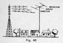
into the ear. A "reflector" is like the back-board on a basketball basket, which prevents the ball from going past the basket and sometimes bounces the ball back into it.
