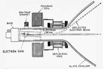
Fig. 21—The electron beam would travel straight ahead to the screen, making only a bright spot, but it is pulled from top to bottom and from side to side by electric currents in the deflection yoke.
