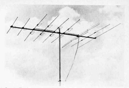
Fig. 45---The element to which the lead-in is connected is called the "driven element." Between it and the TV station are directors, while behind it is the reflector.
