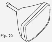
The difference is that, for one thing, the picture tube is much bigger and its purpose in life is to be seen (but not heard). On the inside of the face of the tube is a coating of a phosphor which, when "excited" by a beam of electrons, fluoresces—which is a fancy way for saying that it lights up. If the electron beam can be properly controlled, we will get a picture.
