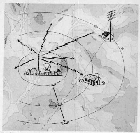
Fig. 35—The strength of the signal determines the type of antenna: inside circle is "close in," second circle is medium range, third circle is fringe area.
