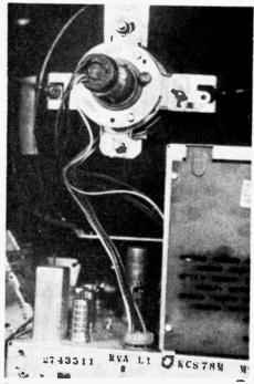
Fig. 31—The socket for the picture tube is usually loose on its wires and is supported by being plugged onto the picture tube base.
