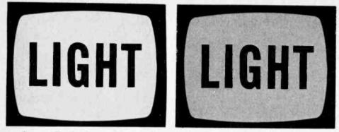
Fig. 7-The Brightness Control affects the brightness of the picture's background
