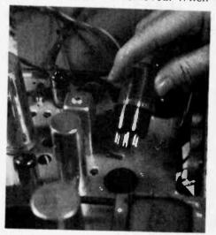
Fig. 27—Octal tubes have a locating pin on the bottom which helps to seat them properly in their sockets.
