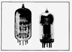
Fig. 19—Miniature tubes are smaller, have no bakelite base. The pins, or prongs, are set right into the glass.
