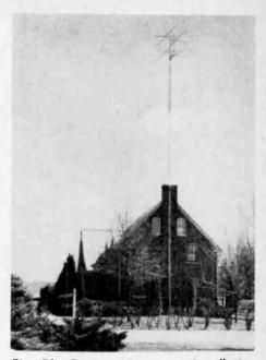
Fig. 52—Typical tringe area installation with 2-bay conical and high, guyed tower.
