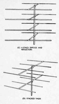
4-stack (or 4-bay) dipole-reflector combination, stacked Yagi's, etc. Practically any type of antenna can be stacked, and to any number of bays, although special design data are needed to do this. In other words, you wouldn't want to try it yourself but you can buy antennas for which someone else has already figured out the problem.
