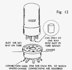
are places to connect wires and other parts which connect the tube into a "circuit."
