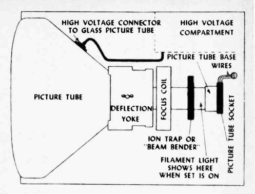
Fig. 30—Typical view from top of chassis, showing placement of yoke, focus coil, ion trap and high voltage connection. In removing picture tube, the high voltage connector and the tube
