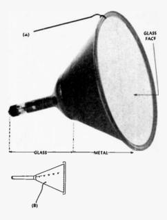
Fig. 28—Metal cone picture tube/High voltage may be connected to the lip (A) or to a snap fastener on the plastic sleeve which covers the metal (B).
