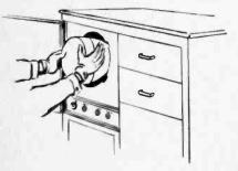
Fig. 29—Removing the picture tube. 36
