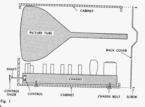
Fig. 3—The back cover must be removed to get at the tubes inside the set. The "AC interlock" disconnects the electric power from the set when the back is removed.
