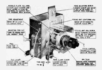
Fig. 32—Alternately turn and slide ion trap along picture tube neck for maximum brilliance of raster. Adjust P.M.
