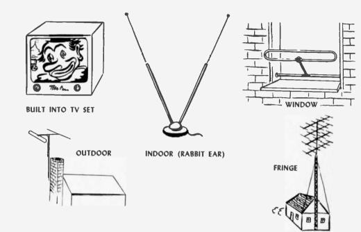
Fig. 38—The strength of the signal in your locality will determine which of these five antenna types will work for you.
