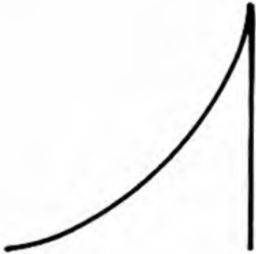
Fig. 2-5. FET transistor exponential response curve.
