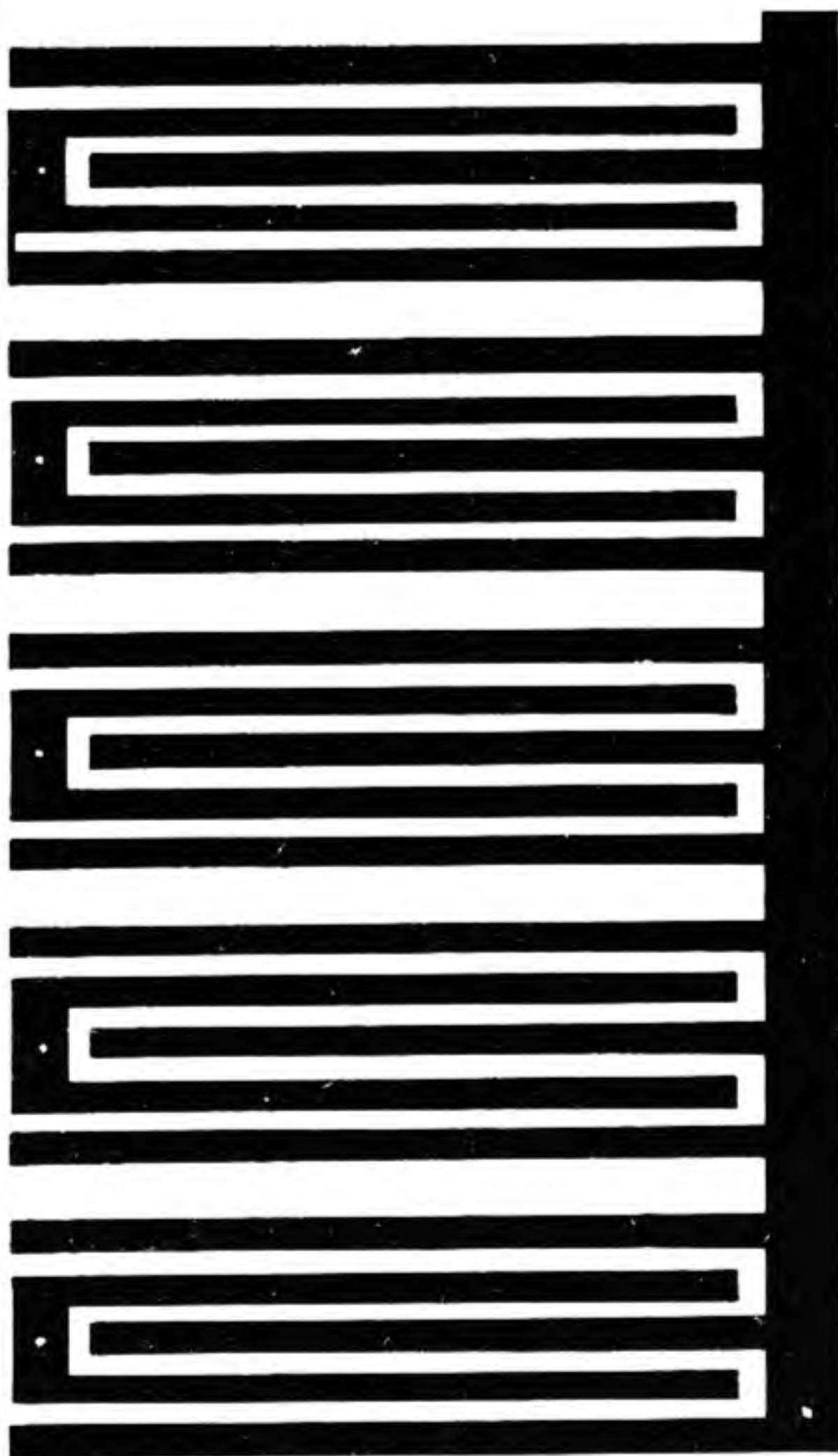
Fig. 7-12. Keyboard foil pattern.
