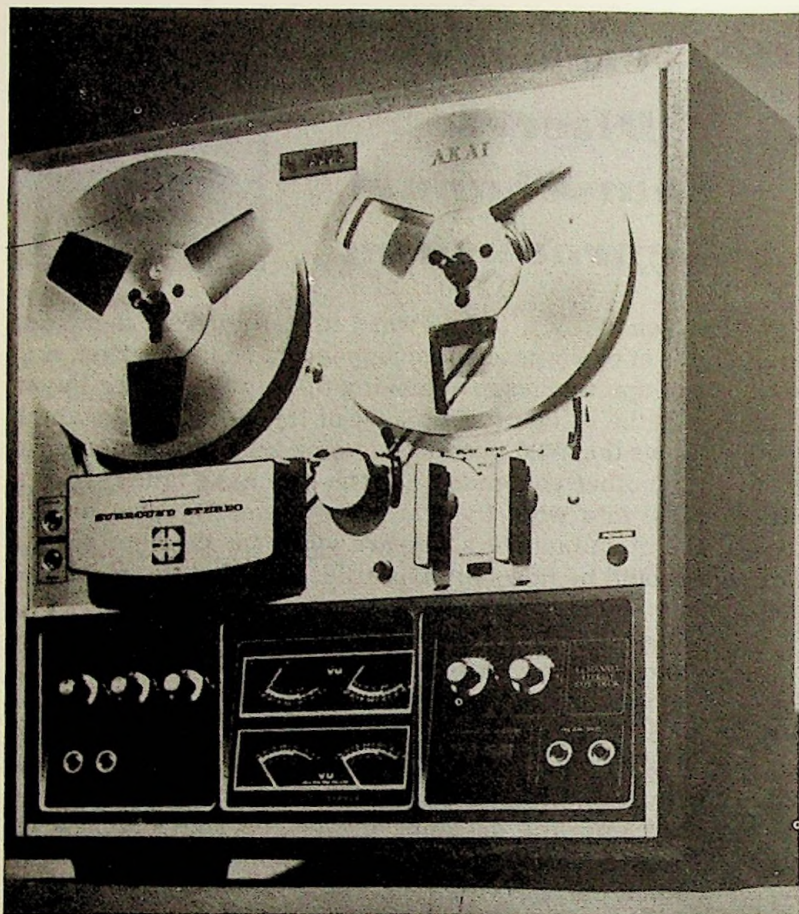
Fig. 5-1. Four channels can be easily handled by tape units, which can handle either discrete signals or four matrixed channels on two tracks.
