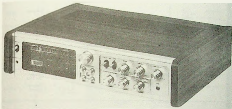
Fig. 9-13. Sanyo's DCX 3000K is a sensibly priced answer to quad. The unit synthesizes, decodes Sansui and SQ. Blend controls allow adjustment of spatial presence. Includes four complete preamps and amps, quality receiver, and sells for $220.
