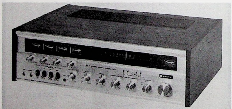
Fig. 9-6. Sanyo's DCX-3300K has three matrix decoders (Sansui, synthesis, and SQ), four metered amplifiers, and a receiver with jacks for discrete operation.
