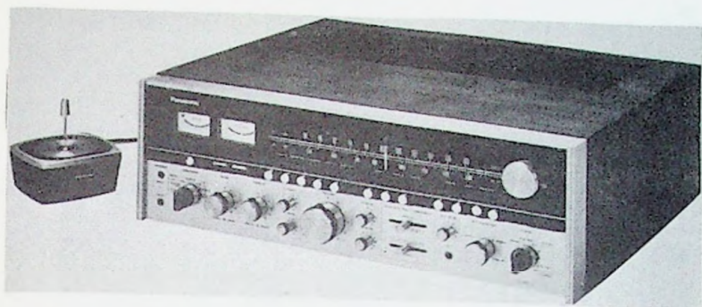
Fig. 9-7. Panasonic SA-6800X includes a very sophisticated four-channel synthesizer for use with conventional stereo records as well as 300 watts of audio.
