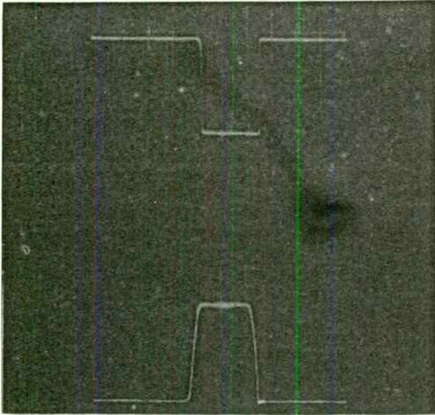
Fig. 6. Output waveform of the circuit in Fig. 5 for minimum pulse width. The sweep speed of the oscilloscope is 1 usec per division.
