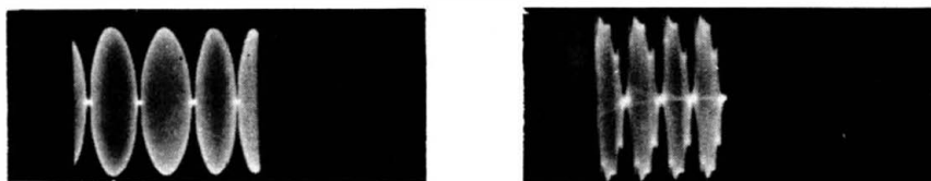
Fig. 11-6. Envelope changes with receiver tuning due to incidental fm.
