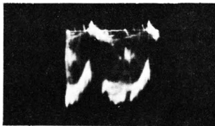
Fig. 4-14. Sync pulses compressed.
