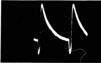
Fig. 6-9. Waveform at point B when C3 is open.
