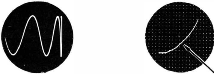
(A) Severe horizontal nonlinearity. (B) Nonlinear amplification present.
