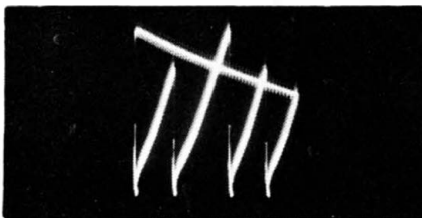
Fig. 10-8. Alternate peaks of the signal have different heights.
