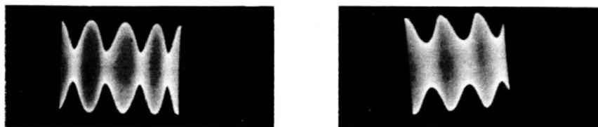
Fig. 11-7. Envelope variation at lower-percentage modulation.
