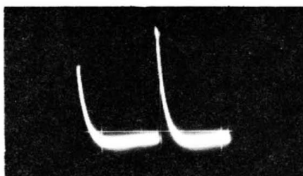
Fig. 8-6. Waveform at point D when C1 is low in value.
