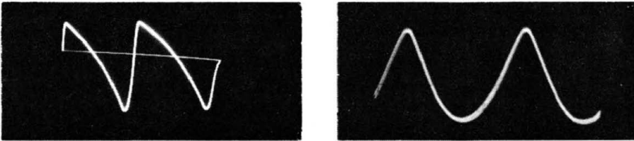
Fig. 10-4. Typical waveforms at filter input.
