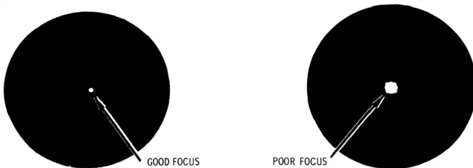
Fig. 2-4. Action of focus control.
