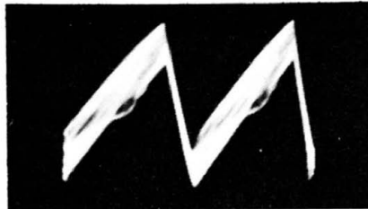
Fig. 6-5. Waveform from horizontal-oscillator circuit when coupling capacitor is leaky.
