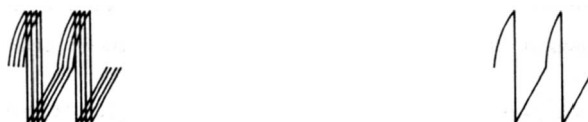
(A) Waveform obtained when unshielded test leads are used. (B) Waveform obtained when shielded direct probe is used.
