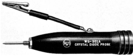
Fig. 4-28. This crystal diode-detector probe is slipped over the regular d-c isolation probe for which it was designed.
