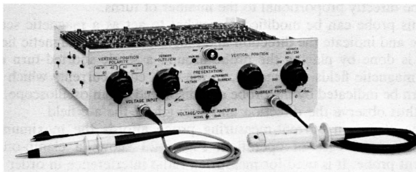
Fig. 6-21. Clip-on probe and amplifier for use with an oscilloscope.
