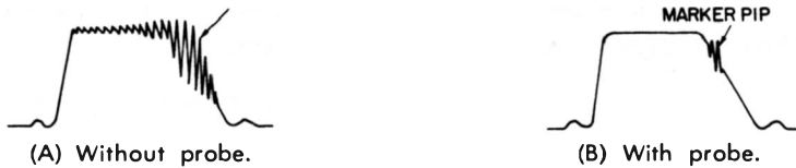
Fig. 1-7. The effect of a resistive isolation probe on the sharpness of the marker pip.
