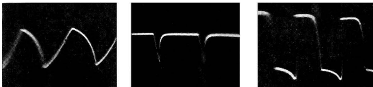
Figs. 9-15, 9-16, 9-17, left to right. Examples of multivibrator output. The wave shape depends on the circuit constants.
