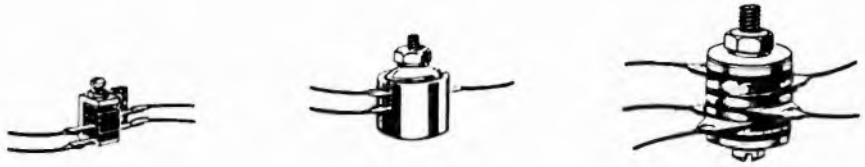
Fig. 6-1. Typical copper oxide instrument rectifiers.
