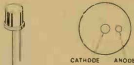
FIGURE 3 Miniature LED with diffused lens. This LED is compatible with most TTL and transistor circuits. It features a Fresnel lens design.
