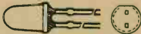
FIGURE 11 This is a high-brightness red LED. It is many times brighter than ordinary LEDs, yet still runs cool.
