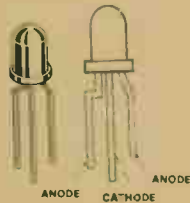
FIGURE 10 This is a jumbo red LED. It consists of two LED elements connected cathode to cathode in a 10mm diameter housing.
