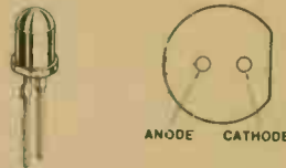
FIGURE 6 Subminiature LED with diffused lens. This device has solid state reliability and is compatible with most TTL and transistor circuits.
