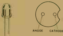
FIGURE 4 This device is a jumbo LED with a diffused lens. It can be used in applications such as pilot and indicator lamps.
