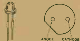
FIGURE 3 This LED features a frosted diffused lens in a plastic encapsulant. When the device is on, it appears as a large, soft light source, making it ideally suited for front panel applications.
