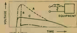
A: Original surge waveform B: Clamping voltage using gap type arrestor C: Clamping voltage using ZNR τ: Discharge lag
