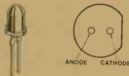
FIGURE 5 Subminiature LED with diffused lens. This device has solid state reliability and is compatible with most TTL and transistor circuits.
