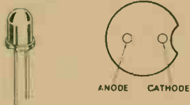
FIGURE 5 This device is a jumbo LED with a diffused lens. It can be used in applications such as pilot and indicator lamps.
