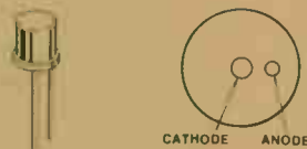
FIGURE 2 Miniature LED with diffused lens. This LED is compatible with most TTL and transistor circuits. It features a Fresnel lens design.
