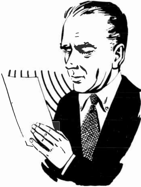
Fig. 1-8. Speaking directly to a sheet of paper causes it to vibrate just as the diaphragm of a microphone does.
