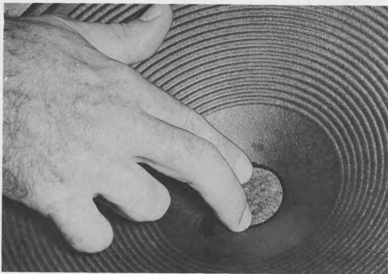
Fig. 9-2. Checking for an off-center voice coil.
