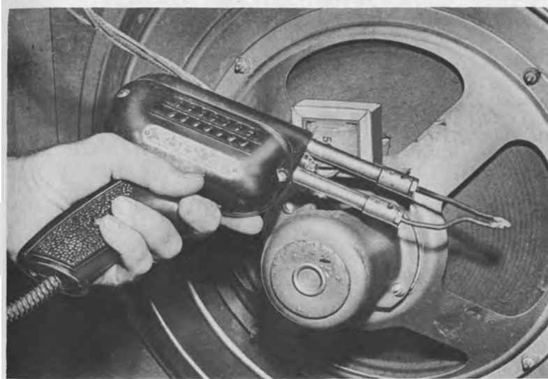
Fig. 2-2. Using a solder gun to check the output transformer and speaker.
