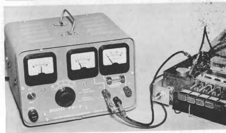
Fig. 14-2. Using an auto-radio battery substitute that has the extra filtering required for hybrid and transistor receivers. (Courtesy of Electro Products Laboratories.)
