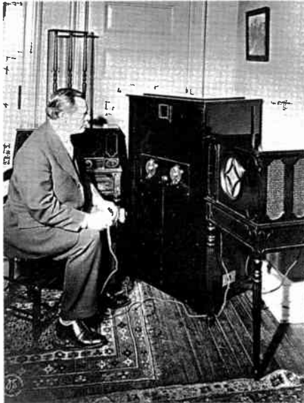
The typical mechanical television set of 1928 was very large, but produced only a small image. Note separate loudspeaker.
