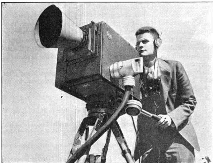
FIG. 19.25.—Portable Iconoscope Camera Used with Mobile Television Unit (courtesy of NBC).
