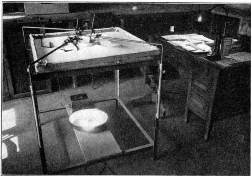
FIG. 3.8.—Rubber Model for the Study of Electron Paths.
