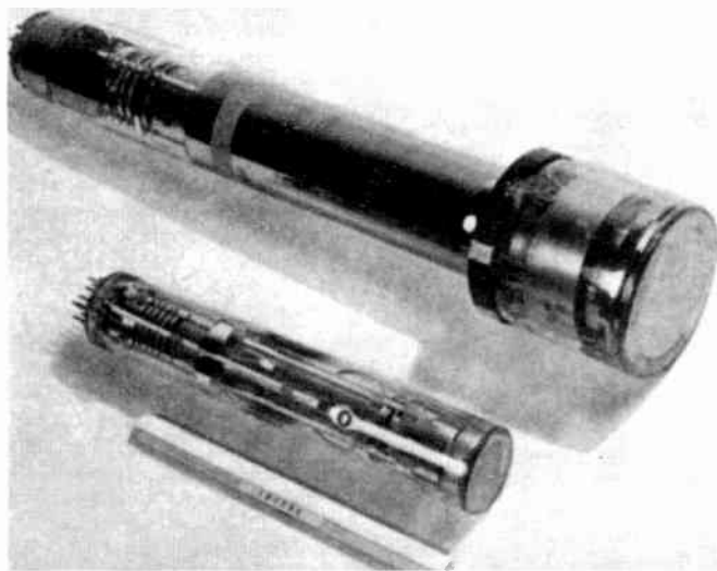
MIMO with image orthicon. Ludwell Sibley photo.
