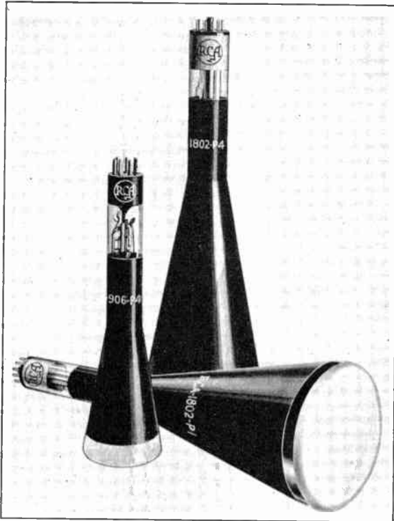
FIG. 12.20.—Small Viewing Tubes Suitable for Television Purposes (RCA 1802-P4, RCA 1802-P1, RCA 906-P4).
