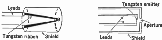
FIG. 13.8.—Two Forms of Demountable Cathodes.
