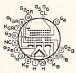
K ULTOR = G_5 + G_6 + CL FOCUSING ELECTRODE = G_3
