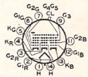
L ULTOR = G_4 + G_5 + CL FOCUSING ELECTRODE = G_3
