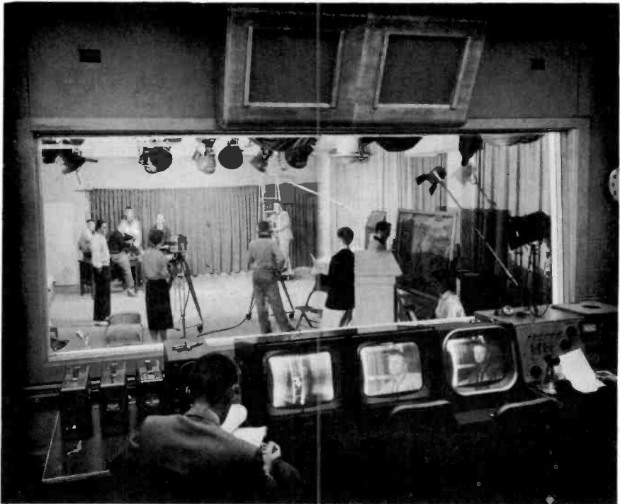
Fig. 8-9. Studio View from Control Room at Northwestern University, Showing Mixture of Ceiling and Floor Lights.
