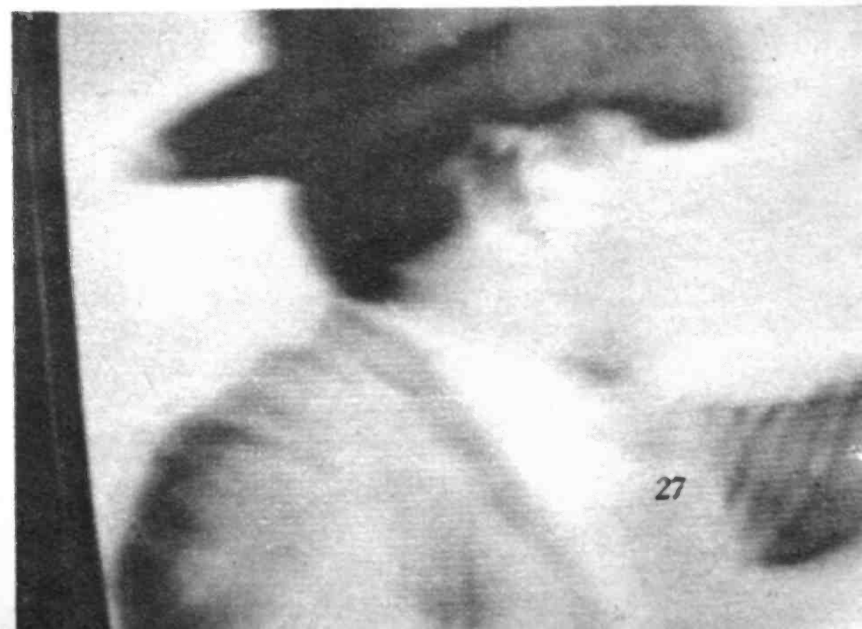
Defocusing is not a common monochrome problem but it happens quite often in color high voltage.
