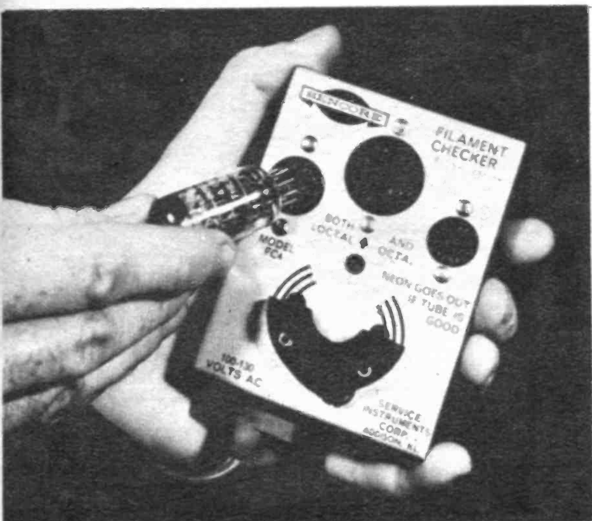
If you own a heater tester now's the time it becomes most useful. The test locates the bad tube.
