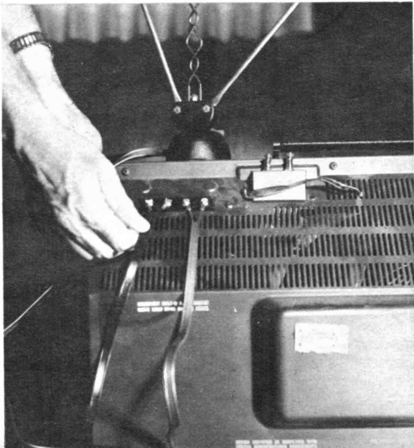
The quick test to determine whether the trouble is in the outdoor antenna is made with rabbit ears.
