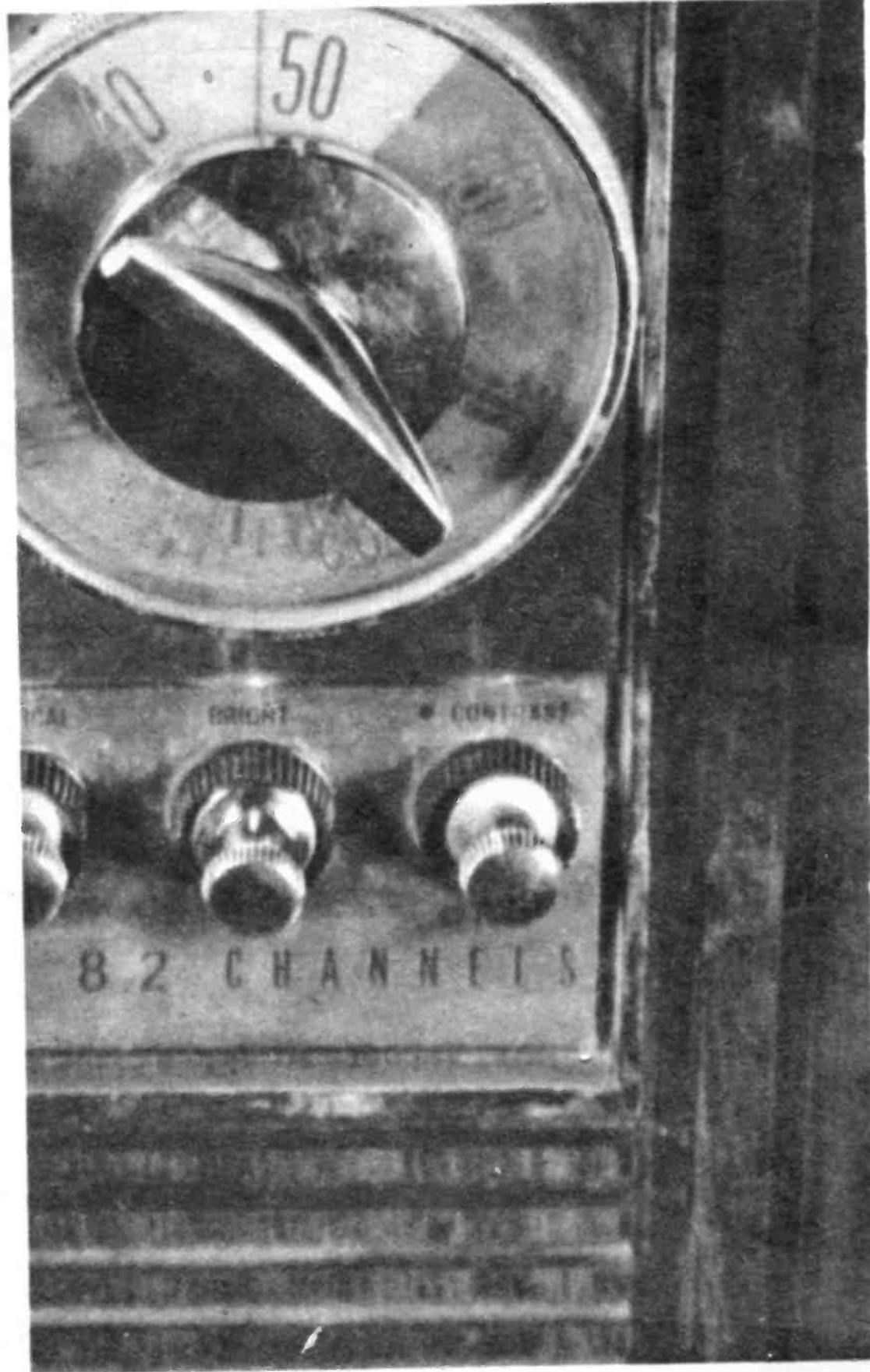
On this particular set the color tint is a dual control in combination with the brightness knob.
