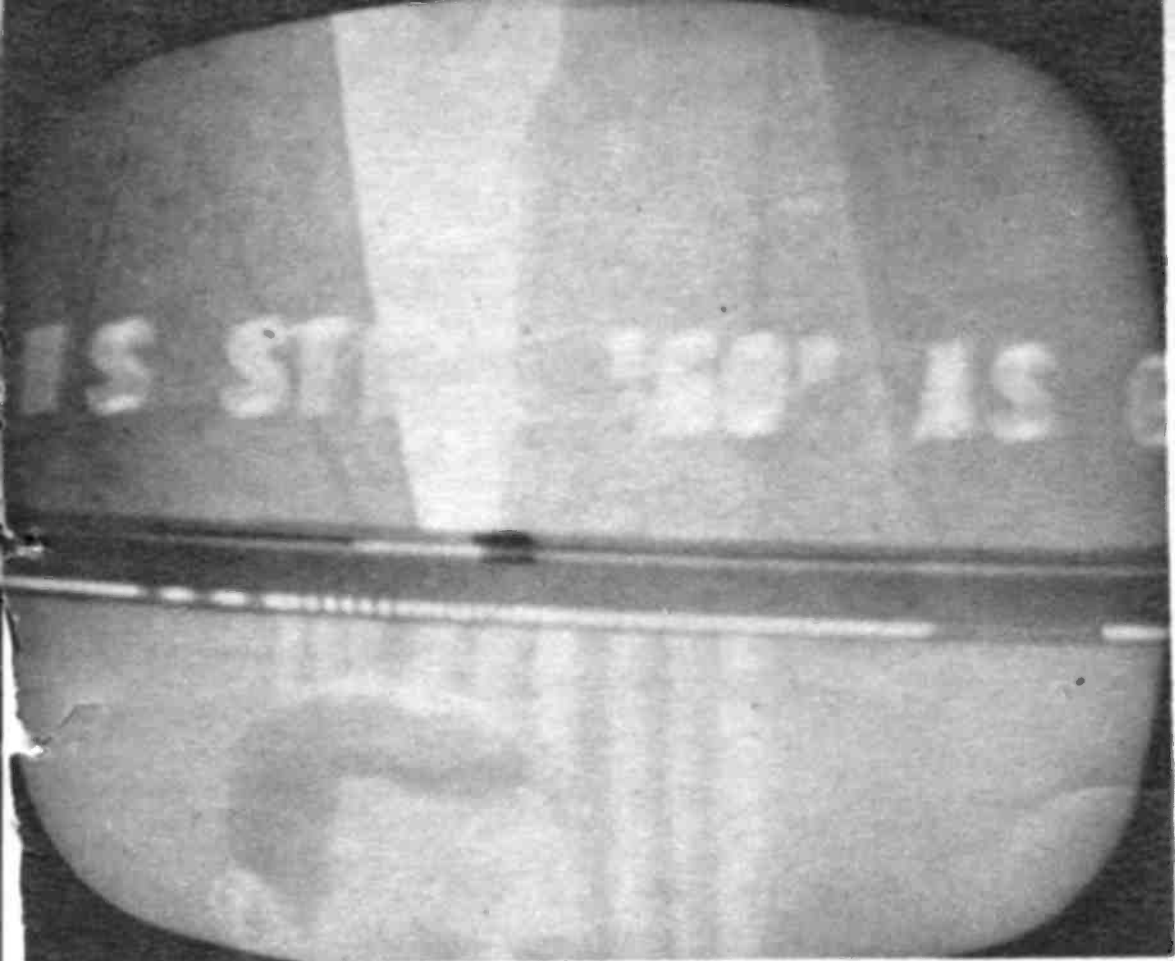
The TV picture can slip down, roll up or whirl past. Either way the trouble is a vertical one.
