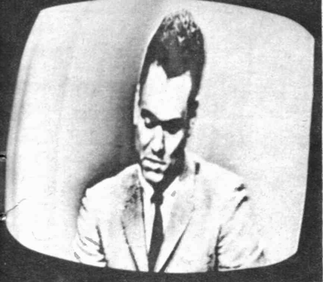
There are many degrees of this two sided shrink condition. As shrink increases, brightness dims.
