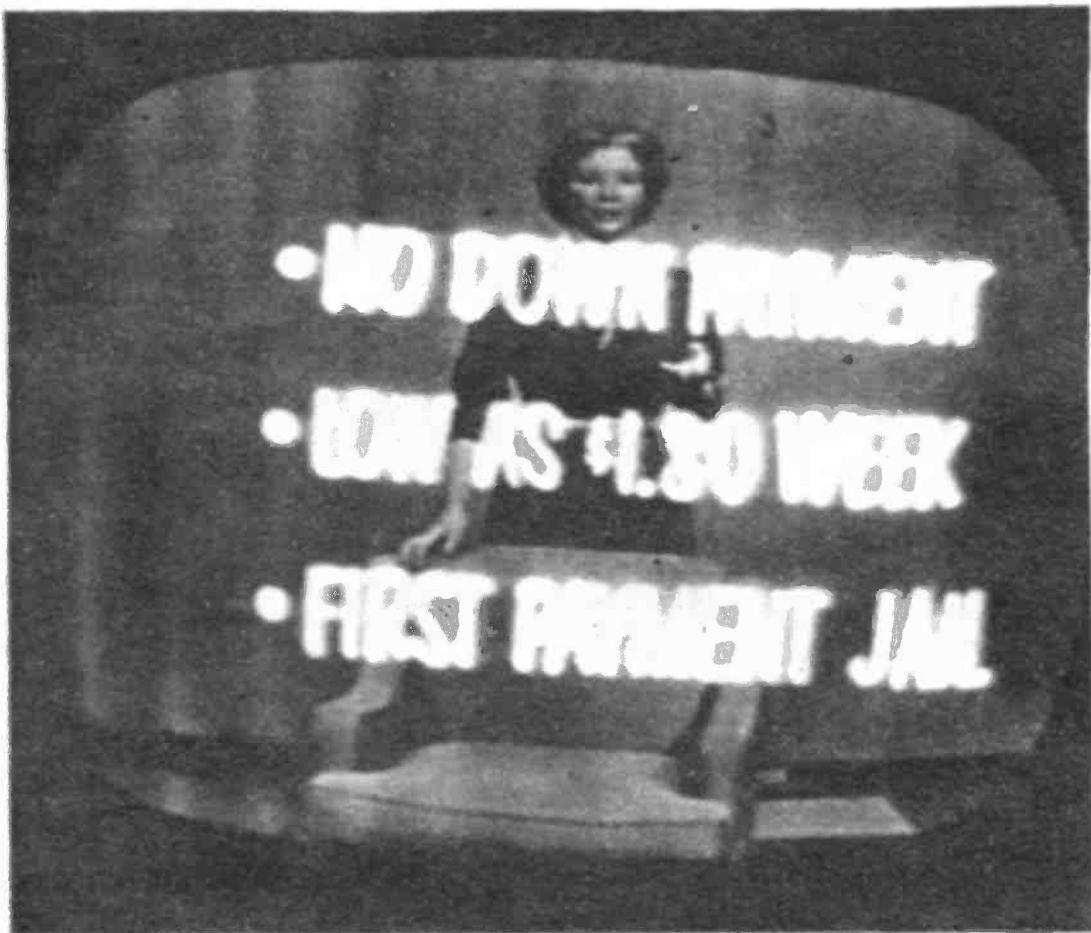
When you replace a yoke and your picture is like this, you must reverse leads in order to restore.
