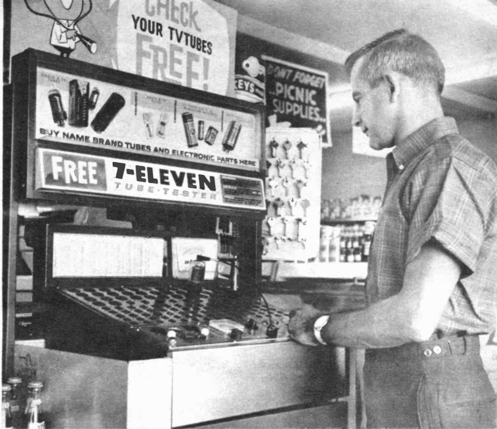
Tube tester found in many stores guides you to the troublesome circuit and the defective TV part.
