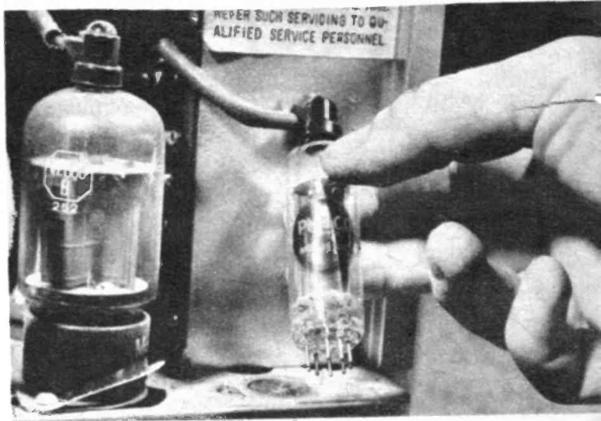
Be careful when removing caps from high voltage tubes. Male and female parts corrode, can crack.
