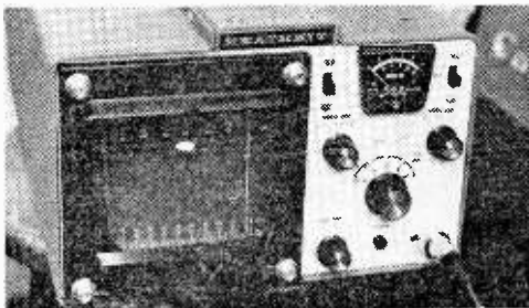
Heathkit ignition Analyzer CO-1015 displays ignition system waveforms on CRT screen. Optional 12-volt inverter (right) fits on back of analyzer.
