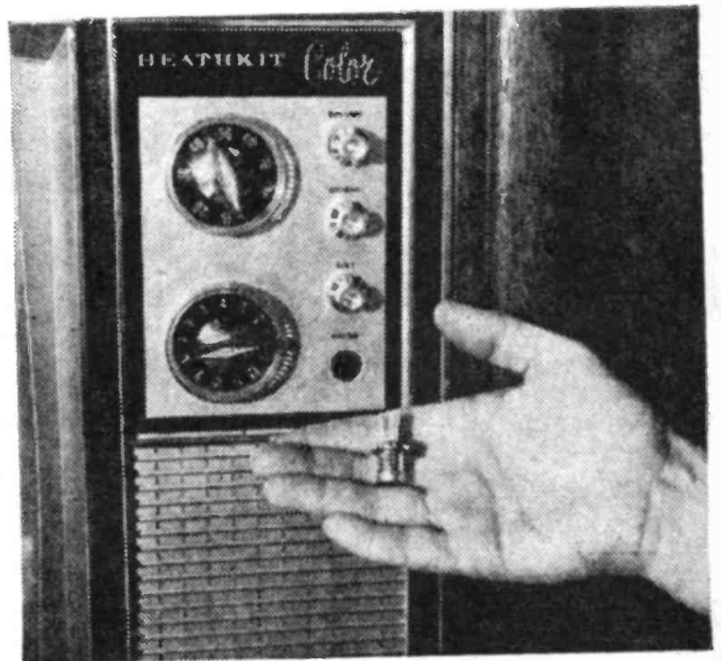
Fig. 2. Lack of color can be caused by incorrect setting of color killer control. On set above, this control is accessible after removing color knob though most sets have control on rear apron.
