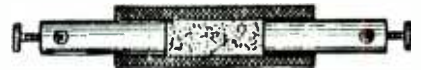
Fig. 1. The Branly coherer consisted of loosely packed coarse metal filings between two metal plugs in a non-conducting tube.
