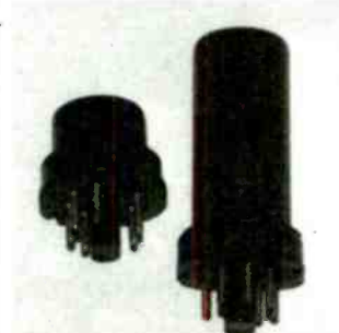
Fig. 7. In the mid-1930's, octal tubes became available. Some versions were glass-envelope tubes, while later versions were metal-envelope types.
