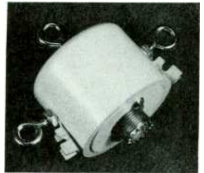
Fig. 5. This type of center insulator has crimp-on lugs for a good electrical connection. These center insulators sometimes contain BALUN transformers.
