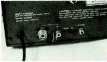
Fig. 8. The rear panel of this shortwave receiver can accept coax, lug-terminal, or bare-wire download terminations. In a pinch, a banana plug could be pushed into the 50-ohm socket for single-wire antennas.
