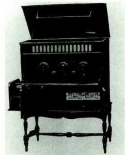
Special radio furniture was designed to provide storage for the early battery set, its power sources and the other accessories required for its operation. Such furniture can be used to display the most prized items in your collection.
