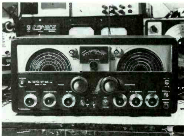
Fig. 4. By the mid to late 1950's, receivers such as this Hallicrafters SX-100 receiver, which used glass-envelope, miniature vacuum tubes, were available.
