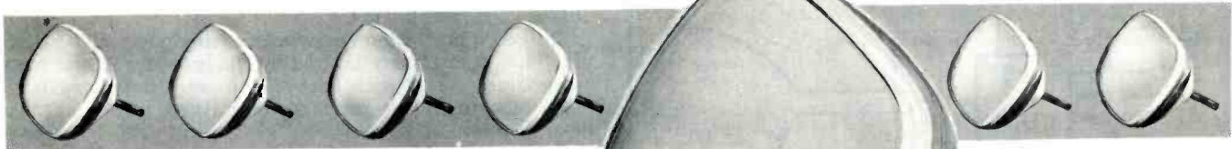
Fig. 1. The Philco color TV picture tube is shown here. The bulb used is conventional.
