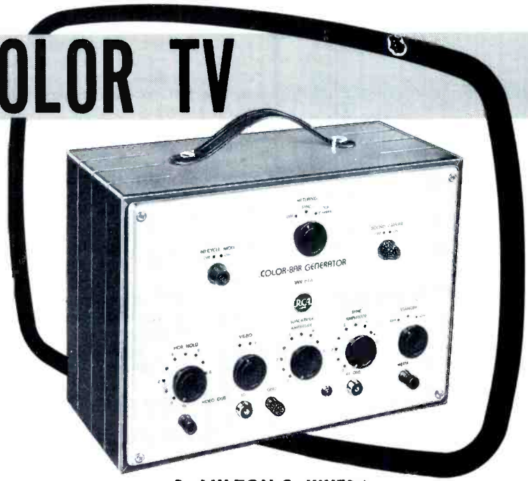
Fig. 1. A color-bar generator is probably the handiest color test instrument. A typical one is the RCA generator shown here.
