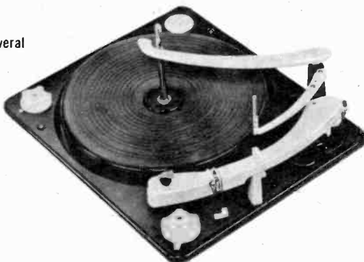
British-built Collaro TC 99 record changer has detachable head, manual-automatic switch
