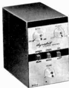
Marantz stereo adapter (at left) and Dyna stereo control (right) provide several functions in addition to ganged volume controls. Each is designed to be used exclusively with manufacturer's preamps. The Dyna unit comes in kit form only
