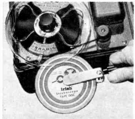
Another accessory is Irish tape strobe disc. With it you can check speed of your tape recorder for complete accuracy
