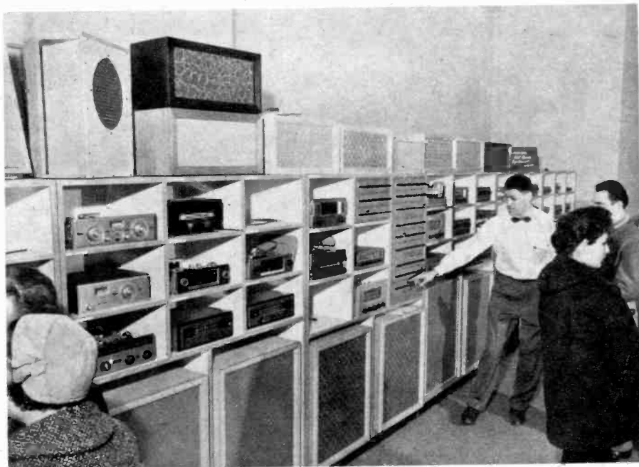
A typical assortment of stereo components is displayed in the showroom of Lafayette Radio, in New York City. The salesman is at a panel of the sort commonly used to switch equipment, so that customers may compare the sound of different items
