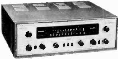
First three-in-ones to make their appearance are Fisher 600 (left), which features stereo 40-watt amplifier; Harman-Kardon TA 230, AM-FM stereo tuner, dual preamps and 20-watt stereo amplifier. These units require only the addition of speakers
