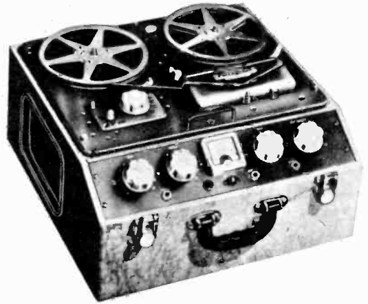
A budget-priced stereo tape deck is the Telectro, at left, which utilizes piano-key controls. Shown on the right is the Ferrograph, a professional portable stereo tape unit that features single VU meter, separate controls for each stereo channel, editing facilities
