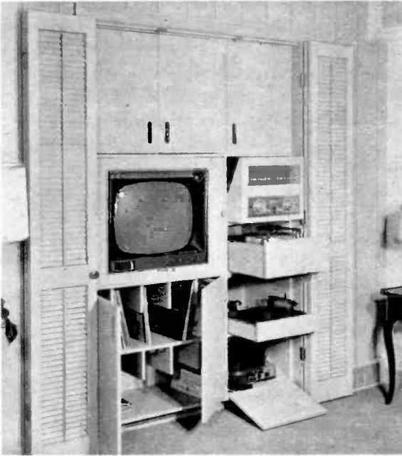
This well-designed, built-in stereo system utilizes a Scott tuner and preamp, J. B. Lansing speaker system, McIntosh basic amp and Rek-O-Kut turntable with arm. Rig looks, sounds good
