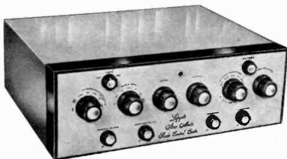
Lafayette Stereo Control has virtually all the controls of stereo preamp on its front panel
