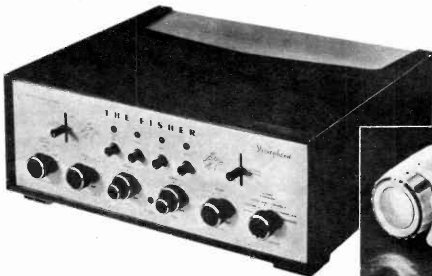
The Fisher Model 400-C is a deluxe preamplifier for stereo, as shown above. It features push button selection of sources, independent tone controls, and an optional remote control unit, above at right.
