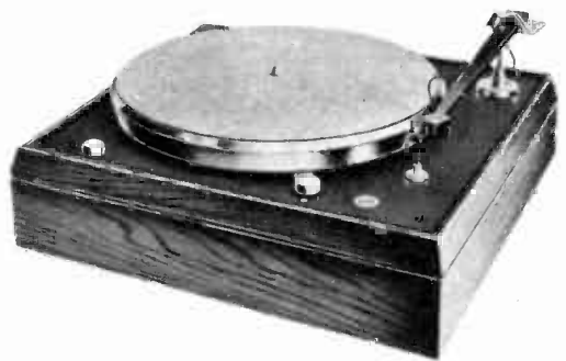
Pickering Gyropoise turntable floats in magnetic field with no mechanical linkage except through very soft drive wheel. The rumble figure is 65 db.
