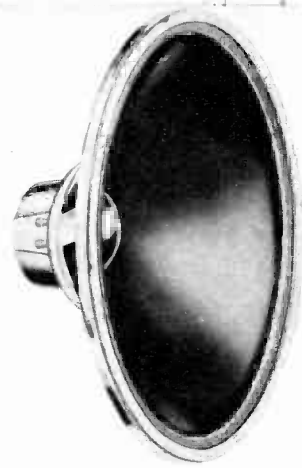
Above is an Electro-Voice 30-inch loudspeaker, capable of reproducing 18 cycles. Cone is molded polystyrene. Used in the Patrician 700 system.
