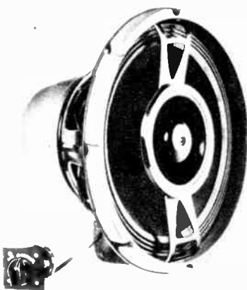
Above, Jensen H-223F coaxial 12-inch speaker with reflexed compression driver tweeter. Below, Vitavox duplex coaxial has 12-inch bass cone, 3-inch hf tweeter; 30-15,000 cps, 30 w. 15 ohm.
