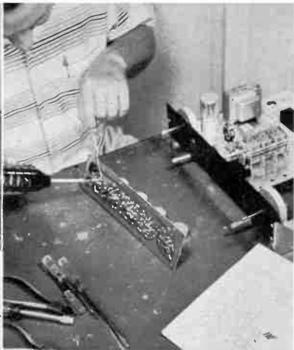
Installation of components on i-f etched circuit board of FM tuner comes next. Using soldering gun, apply solder sparingly to all proper points.
