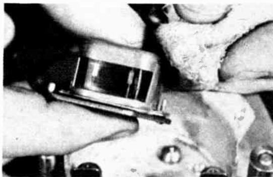
This is photograph of a typical tape erase/playback head, removed from a home tape recorder.
