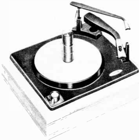
Heathkit record changer comes in kit form, takes G.E. cartridges. It includes 4-pole motor, friction drive, has four speeds and manual operation.
