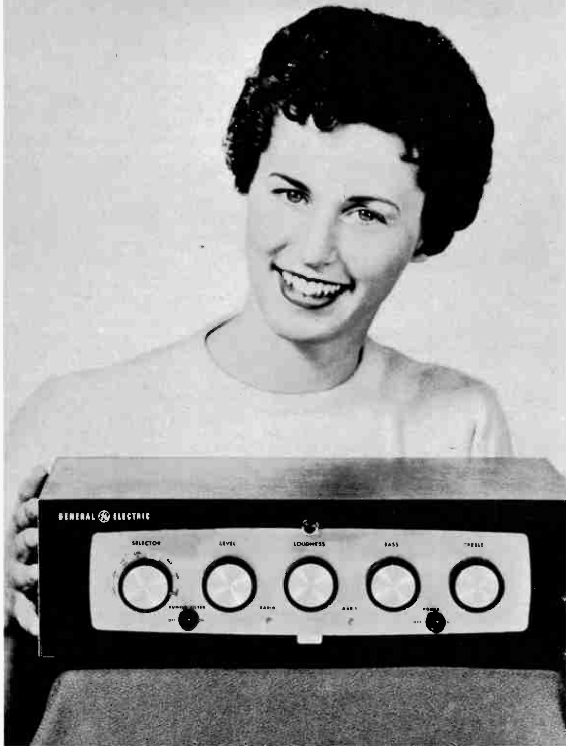
General Electric Model PA-20 control amplifier has 20-watt power output, costs $99.95. Harmonic distortion is below 1 per cent. Phono input hum level is 60 db at full output. Unit contains a rumble filter.
