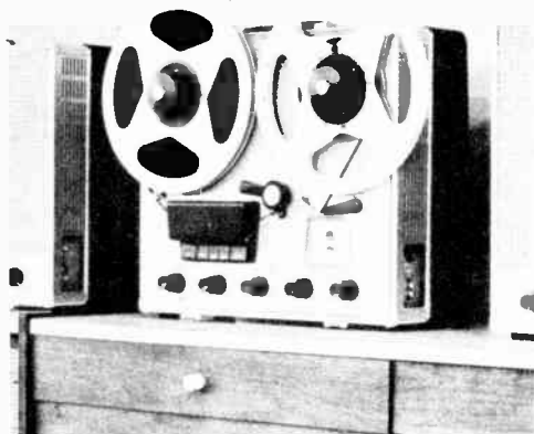
American Concertone "Globematic" 60 recorder has mechanism and preamp, separate speaker.
