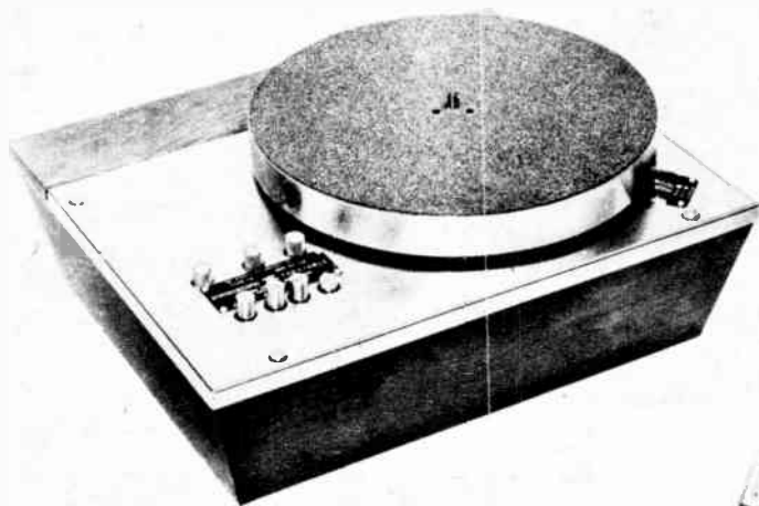
H. H. Scott turntable has push-button 3-speed selection, built-in stroboscope; motor board is stainless steel-covered. Special slip clutch, at right, allows turntable to be cued, avoids drive shock.
