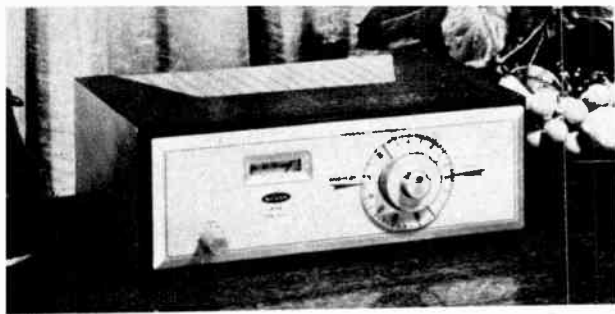
H. H. Scott 311-C FM tuner gives sensitivity of 2 \mu v for 20 db quieting at 300 ohms, 1 \mu v with 72-ohm antenna. Two stages of full limiting and 2-megacycle detector bandwidth are also featured.
