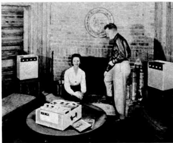
Completely portable stereo system by Bell uses two matched speaker-amplifiers. The tape transport in foreground will play back and record stereo.
