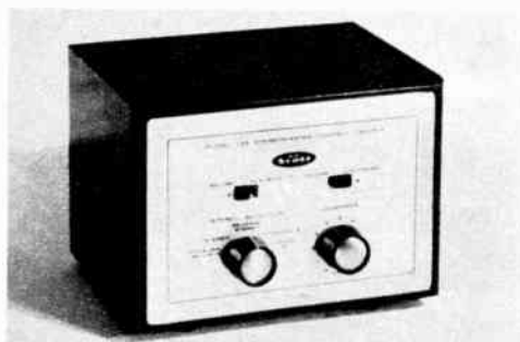
This Scott unit, Model 135 Stereomaster Control Center, combines with a regular preamplifier to give you stereo control for the added channel.
