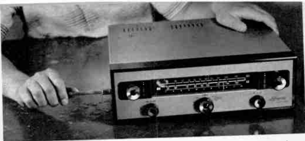
Tuning components of set are previously aligned at factory, but front end touch-up may be done at home. Tuning eye can be used as alignment indicator; when the alignment is completed, tuner is ready.
