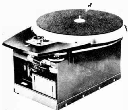
Fairchild Model 412-4 uses synchronous motor, has variable speed with its "electronic drive" unit, which drives the motor at four speeds.
