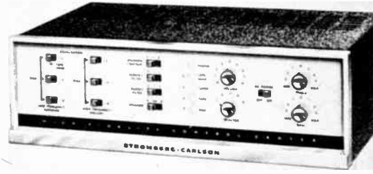
Stromberg-Carlson AR-432 stereo control amp has 30-watt power output, speaker selector, low and high frequency equalization, rumble filter. Response is \pm .9 db, 20-20,000 cps full output; $119.95.
