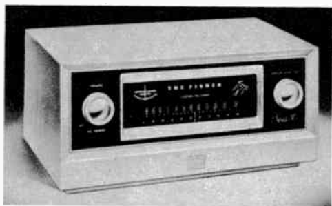
Fisher FM-40 tuner has center-of-channel tuning meter, 3 uv for 20 db quieting sensitivity, 300- or 72-ohm inputs, multiplex, is self-powered. It features logging scale, power/volume control.
