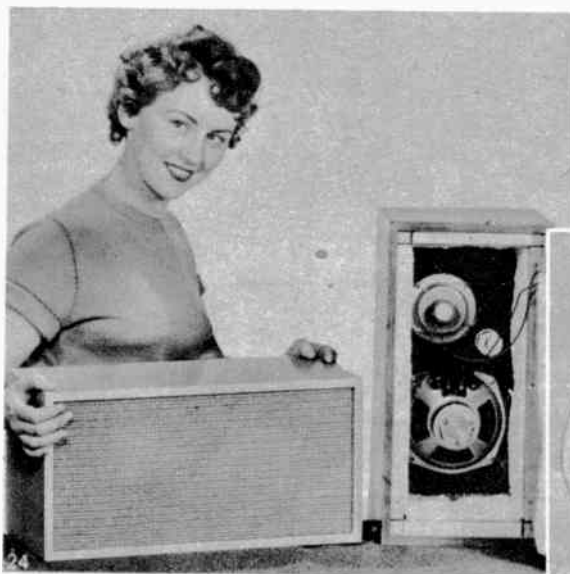
Speaker system package and enclosure kit by General Electric has 6-in. woofer, tweeter, network; \frac{1}{2} cu. ft. cabinet; $49.95-$57.
