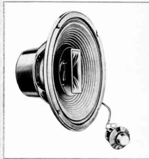
Electro-Voice 12TRXB 12-inch triaxial speaker. $64. Response is 35-15,000 cps. 20-watt capacity. Sensitivity is 46 db.
