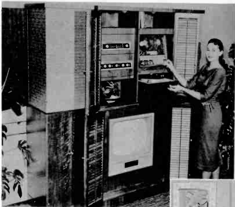
Bell components in custom installation for stereo reproduction include FM-AM tuner, Model 3030 stereo amplifier, tape transport, Bozak speakers.
