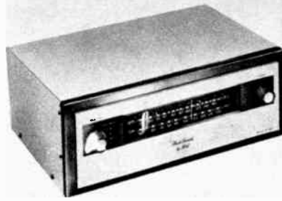
Fisher FM-AM tuner and audio control Model 90-T. FM sensitivity: 0.85 uv for 20 db quieting, 1.6 uv for 30 db. Audio control has eight-position channel selector, record and tape equalization.
