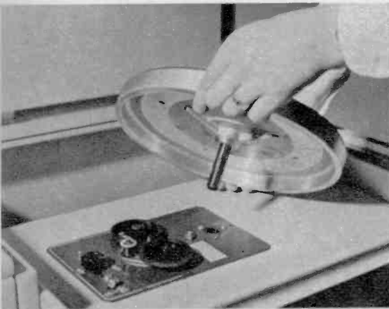
Motor is screwed to board and then turntable is installed. Power wire runs through drawer bottom.
