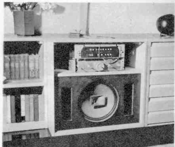
Note slots on each side of coaxial speaker. These were designed to give proper bass reflex response.
