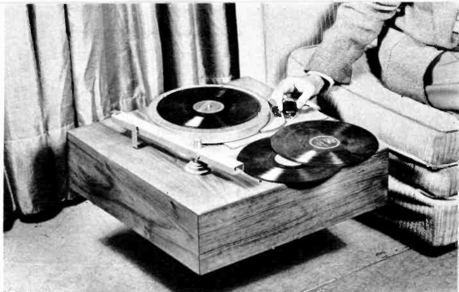
The home craftsman can easily build a custom mounting for his turntable assembly. No automatic changer is needed if records used are predominantly long-playing type.
