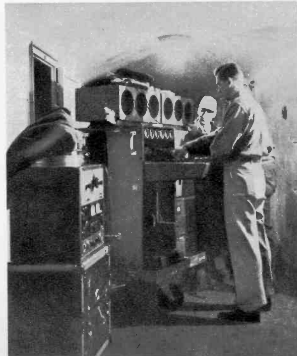
Technicians for Cinerama must monitor six separate sound tracks to give audience impression of extra dimension of sounds which move and surround.
