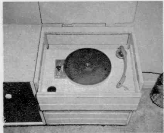
Mounting of pickup arm completes the assembly. Cabinet top was removed, refastened with hinges.
