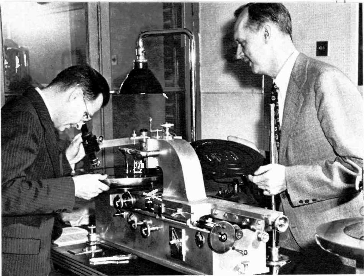
While William S. Bachman, director of engineering for Columbia Records, watches at right, record being cut on lathe is examined by Dr. Peter Goldmark, the man who perfected the 33\frac{1}{3} r.p.m. long playing record.
