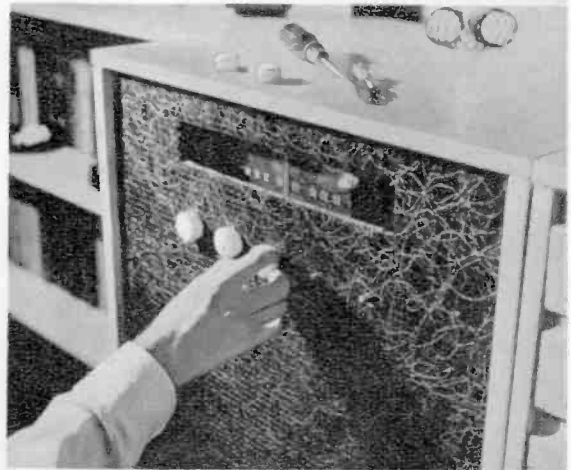
Knobs to match cabinet wood color are now fitted on protruding shafts of the tuner-amplifier unit.
