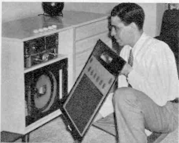
Pressed-wood board with openings cut was covered with fabric and fitted into old sliding-door slot.
