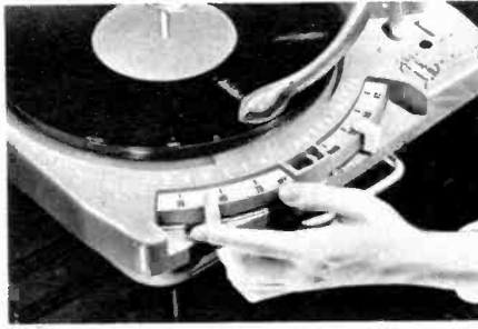
Cobra pickup arm of Zenith players uses a metal vane moves by the stylus to modulate AM radio waves which are locally generated by an r.f. oscillator.
