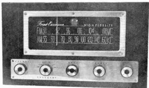
An AM-FM tuner made for high fidelity use is this set by FM pioneer Freed-Eisemann.
