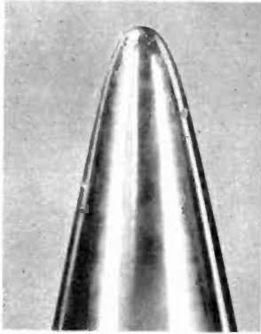
An old-fashioned steel needle tip looks this way before use.
