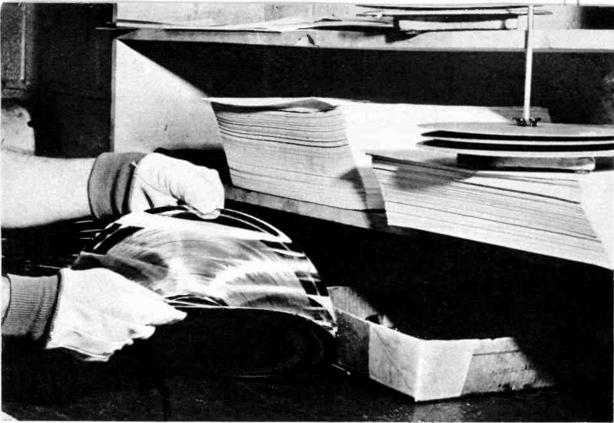
After going through the plating tank process, the stamper is gently separated from lacquer master. RCA Victor photo
