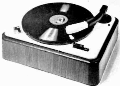
Turntable made by Thorens of Switzerland has a variable speed direct drive motor. Helical gears of sound-absorbing material, plus a special speed governor, makes possible exact 78, 45, or 33 r.p.m.
