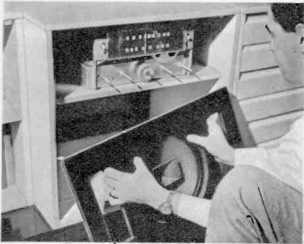
Bottom cabinet space is used as enclosure for the loudspeaker. The mounting board bolts into place.
