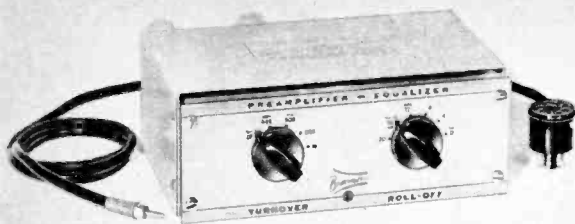
Turnover and roll-off bass and treble positions of the Brociner A-100 pre-amplifier-equalizer give corrections plus magnetic cartridge amplification.
