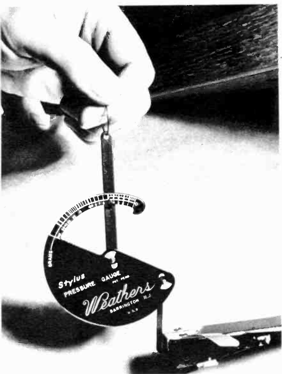
The Weathers stylus pressure gauge, shown testing a Weathers tone arm, is of the balance type. The proper weight directly affects fidelity and wear.
