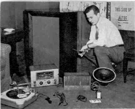
Assembling matched components can be done with minimum tools. Screwdriver joins these Altec units.
