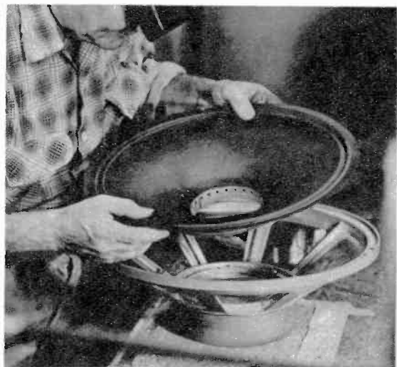
CONE must be microscopically centered, so the craftsman resorts to use of powerful magnifiers.
