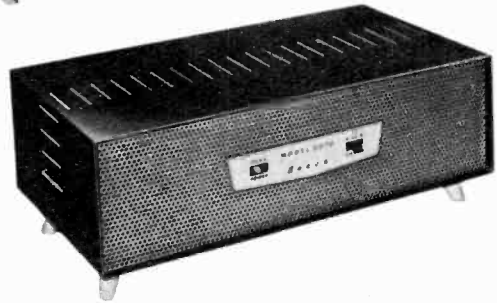
E-V PC-2 music control center, left, provides control for amp, has self-contained power supply.
