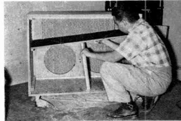
WITH front speaker panel in, wing partition is fitted to separate three speakers' sound chambers.
