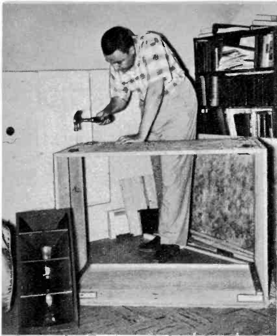
VENEERED-PLYWOOD box is first constructed as author Hoefler shows. Drawings which clarify each step are reproduced from kit's instructions.
