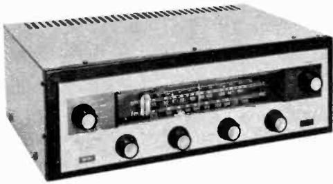
PILOT HF-30 is a medium-powered FM-AM tuner, preamp-equalizer, 12-watt amplifier in metal case.
