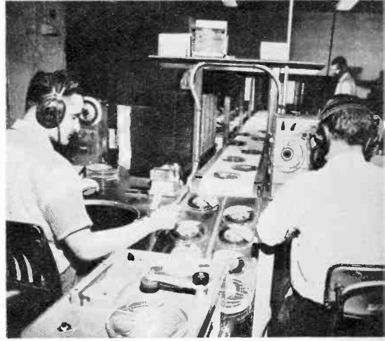
CONVEYOR carries the stereo tapes to testers, foreground, who make selective tests of output.
