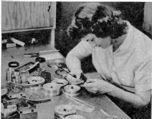
ASSEMBLY of diaphragm for high-frequency unit of JBL speaker is intricate and painstaking task.
