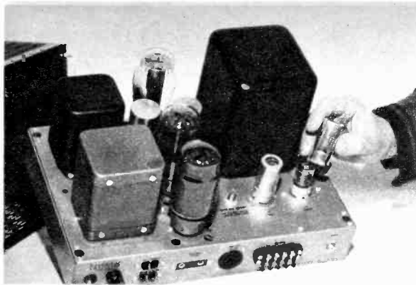
SHIELDS in preliminary stages must be twisted and removed before tubes can be taken out.
