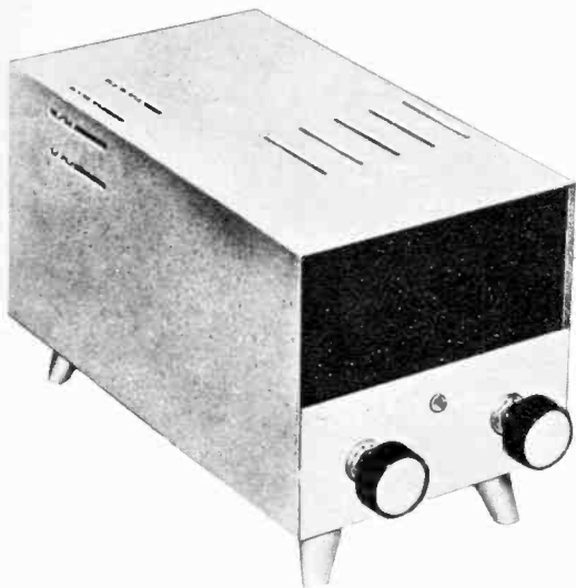
STEREO can be economically added to existing high-fidelity systems with the Bogen ST10. Dual preamp, 10-watt amplifier are in the one unit.
