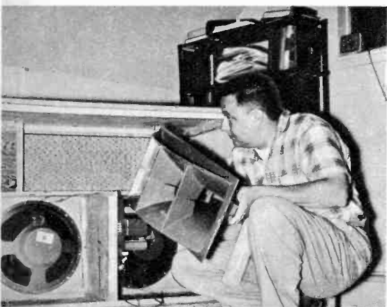
TWEETER UNIT , a sectoral exponential horn, is now to be mounted. You will note that the crossover network is already in, having been attached to the side of the center partition with wood screws.
