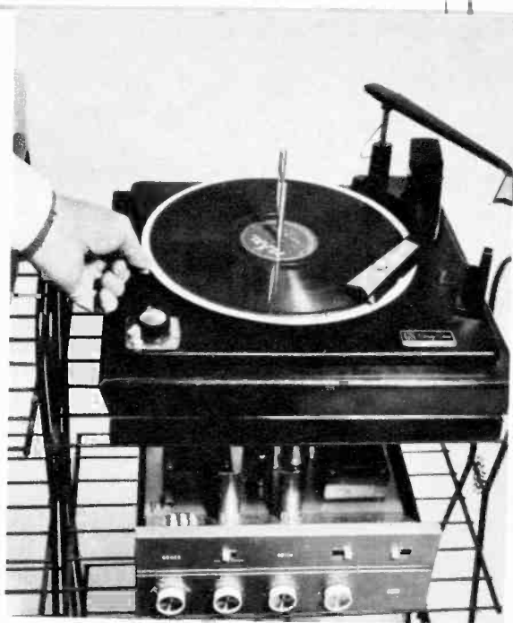
PAPER is held, keeping the record stationary as turntable turns. At proper moment, release paper to start record, bringing music in on cue.
