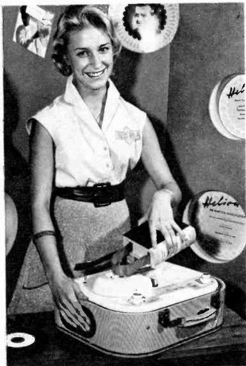
THIS GERMAN recorder takes up to 70 sound tracks on tape that is 1\frac{3}{8} inches wide, or a little over 5 times as wide as the US standard.
