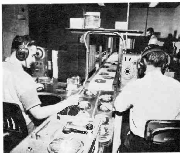
CONVEYOR carries the stereo tapes to testers, foreground, who make selective tests of output.
