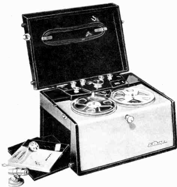
THIS EKOTAPE model is correctly matched for recording from hi-fi, but for direct playback connection to setup, slight modification is needed.
