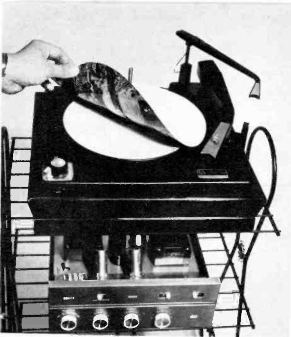
FOR SKIDDING record prior to fade-in, place paper disc between the record and turntable. We used an old photo here, with glossy side down.
