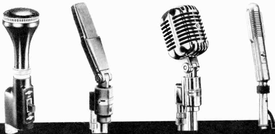
MICROPHONES shown, left to right, are Astatic dynamic type of high or low impedance; Shure multi-impedance, velocity ribbon-element model 300; the Shure 556 dynamic, an old hi-fi standby of multi-impedance; and Fen-tone bi-directional velocity mike which is adjustable to any one of three impedances.
