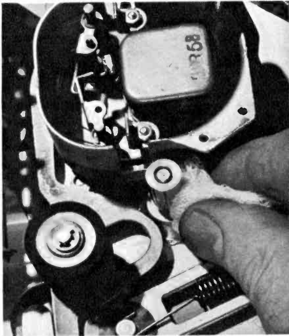
CLEAN CAPSTAN'S surface similarly and dry. Dirt causes uneven tape motion, wow, flutter.
