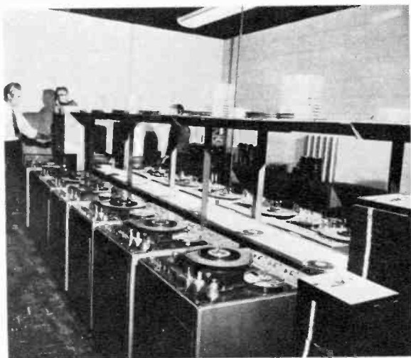
"MASTER" is at the far left; engineer has just pressed button to start "slaves." Note conveyor.
