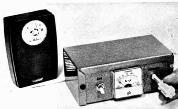
Pager is tuned to an unoccupied spot on the broadcast band by adjusting a front-panel-mounted coil. Radio becomes quiet when Pager is on frequency.
