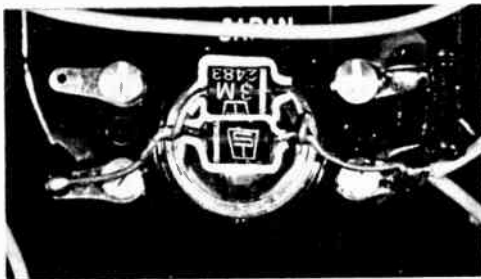
Install diodes (shown here outlined in white) directly across meter terminals in VTVM or VOM.
