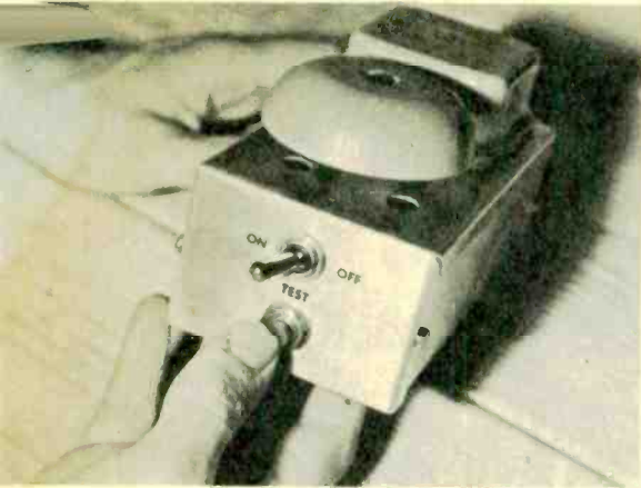
The bell of the wading pool alarm can be tested by installing a simple press-to-test switch unit.
