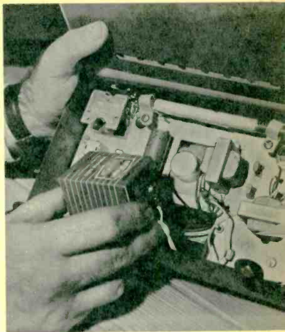
The unit uses a nine-volt battery. Horizontal rod across the top is a self-contained ferrite antenna.
