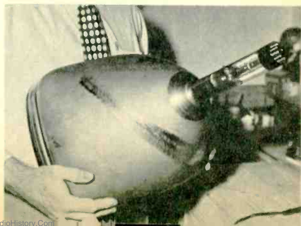
Here is the correct method of carrying picture tube. It should NEVER be held by its narrow neck.
