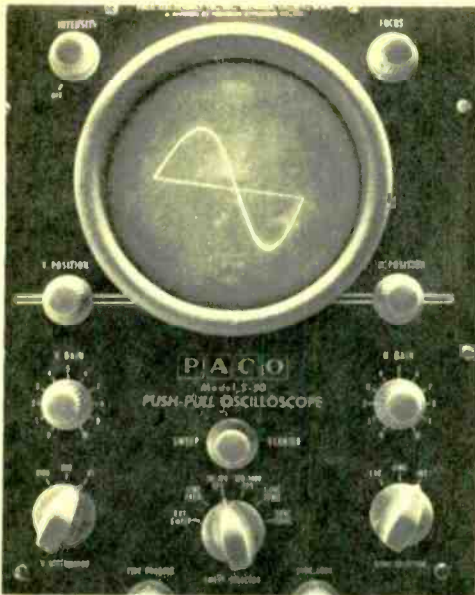
Photo of actual trace of ordinary 60-cycle AC as seen on scope face. This is classic "sine wave."
