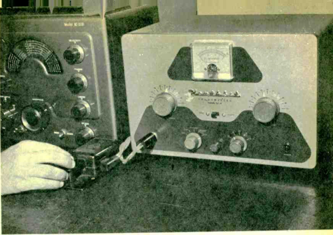
Closeup of completed DX-40, ready for CW operation; key plugs directly into front panel.
