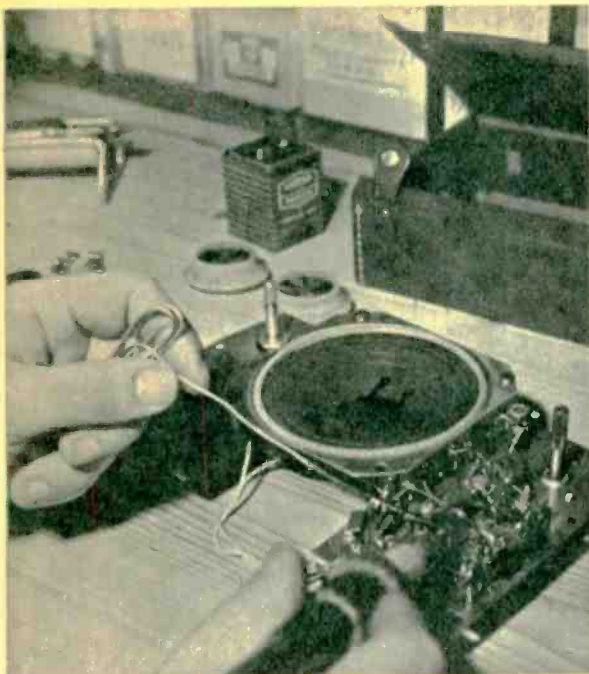
Follow instructions when soldering components in place. Always use rosin core solder, hot iron.
