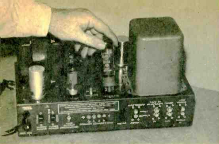
Tube positions are easily identified by callouts. Big transformer at right side of chassis is output transformer, capable of handling 50 watts. Note the various phone jacks and outlets located on the rear panel of the unit.
