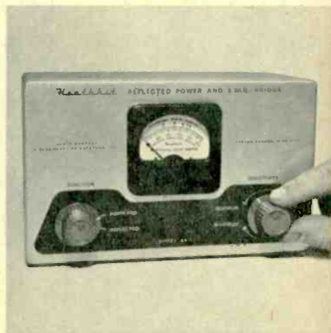
Details of front panel controls of S.W.R. bridge are shown in photo above. Diagram on the opposite page shows circuit arrangement of Heathkit Model BX-1 Reflected Power and S.W.R. Bridge.
