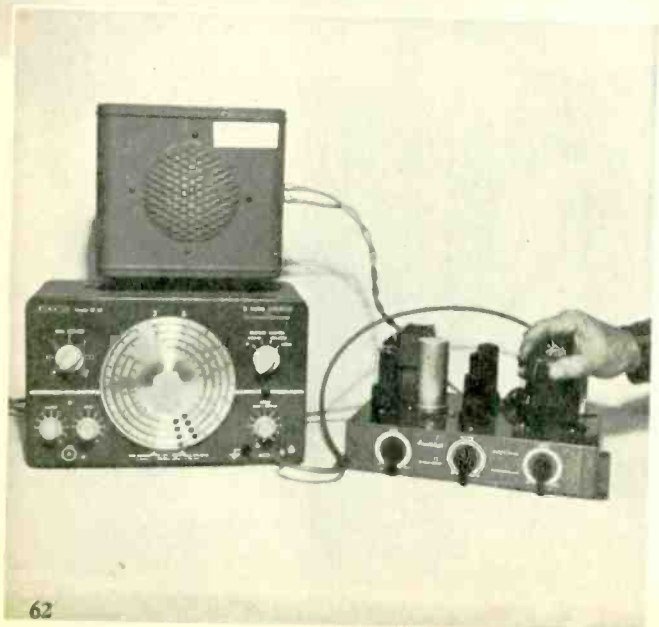
Left, the 400-cycle tone of the signal generator is taken from the connectors at the lower right corner of the front panel, for a test on a small high fidelity amplifier. After testing, a suspected tube was removed and found to be the main cause of trouble.
