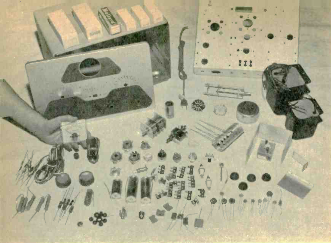
Complete layout of all parts removed from shipping box. Note the neatly punched chassis.
