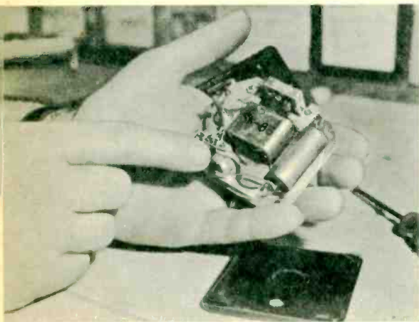
Finger points to small transistor that does all the work. Note the neat design of this kit unit.
