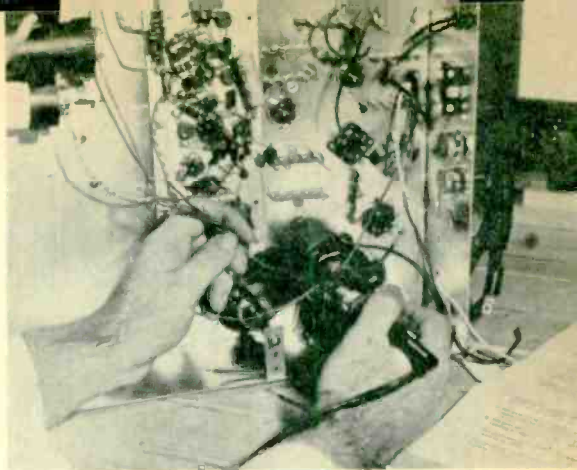
All solder connections must be tight. Allow heat to flow thoroughly before removing the iron.
