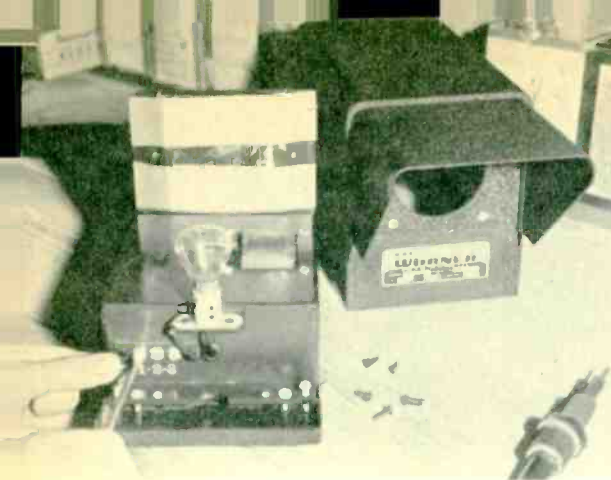
Terminals on the case enable you to make all the necessary electrical connections to light source.
