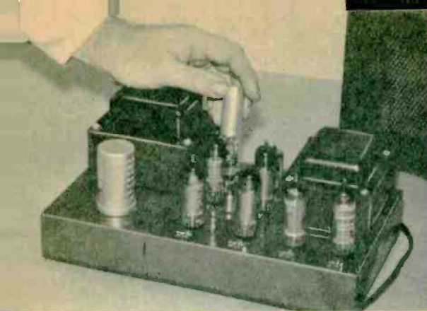
After wiring, place tubes in their sockets. All the tubes, except the 6AV6, are British imports.
