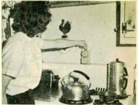
Cut-off switch on alarm bell enables you to have pool in use without bell ringing. See schematic.
