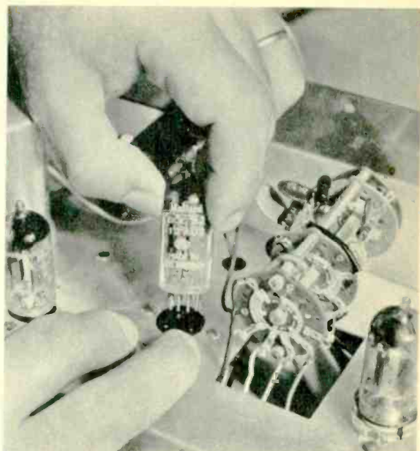
Many of the tubes used are imported from Great Britain. Photo above shows the Mullard ECC-82.
