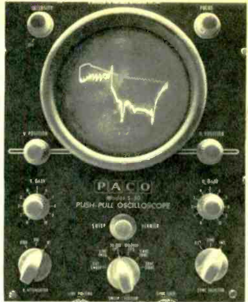
This zig-zag trace was obtained by hanging the vertical input leads near a fluorescent lamp.
