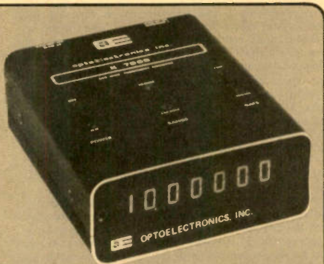
Smaller frequency counters like this one from Optoelectronics, Inc. are all the counter that most hobbyists will ever be in a position to need.
