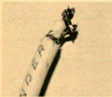
Here's a closeup of the probe assembly. Anode is soldered to the coax center wire.
