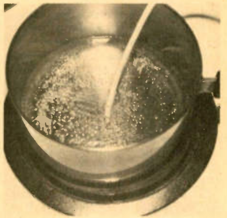
Allow 5 minutes in boiling water to compensate for thermal inertia in the diode.
