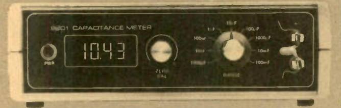
In experiments or projects involving complicated circuitry, it is often important to know the exact capacitance of components; this capacitance meter is the ticket.
