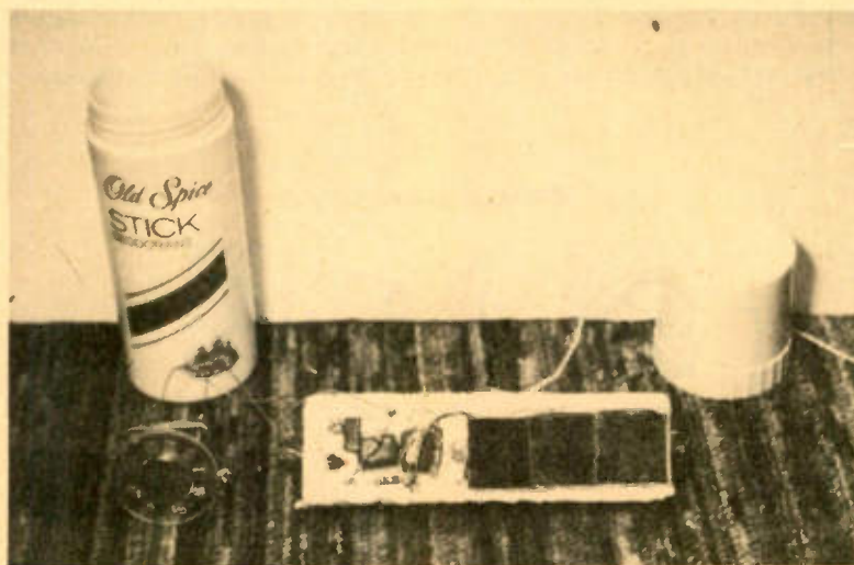
All components are mounted upon a piece of foam 1 x 1 \frac{1}{2} x \frac{3}{4} -inches thick.
