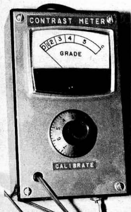
Photograph of Contrast Meter shows its meter calibrated for various paper grades.
