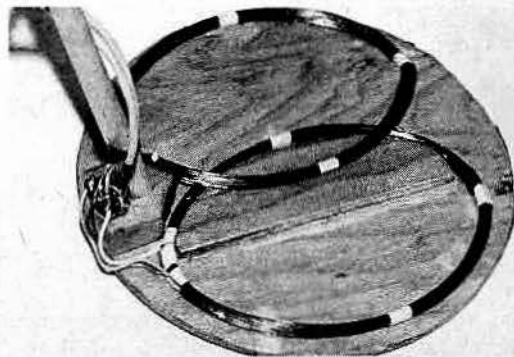
Closeup of the search head shows the position of coils L1/L2 and L3, and their respective overlaps as described in the text.
