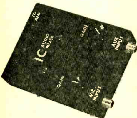
Mini Mix is compact professional looking unit that's easy to build using IC whose tiny "chip" contains circuit at right.
