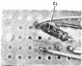
Bottom view of circuit board shows C1 and connections to speaker and B1.
