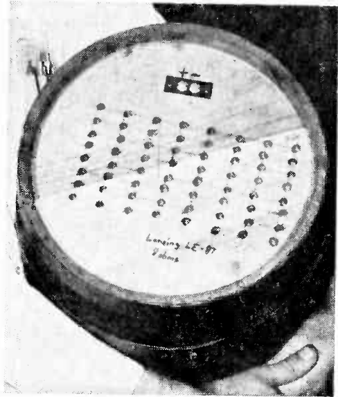
Though the 64 holes in barrel pictured above have been drilled in a neat pattern, this is not essential for good sound. Terminal block is for making connections to speaker.
