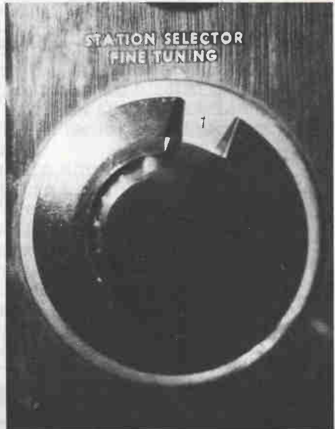
Here is a close-up picture of the tuner from a 1946 TV set, which clearly shows channel "1" on the dial.
