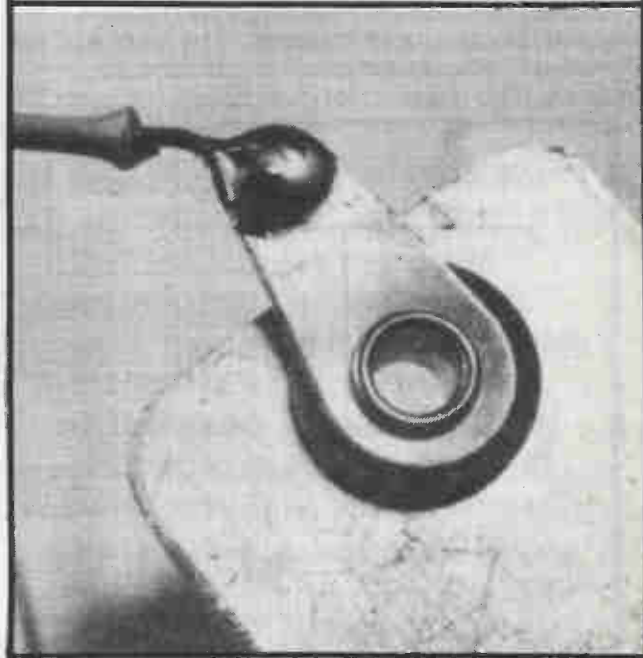
This picture shows a good soldered joint. It has enough solder to hold securely and make a good electrical connection. It has not too much solder, not too little.
