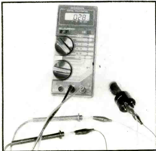
Photo #15. Testing a tube with a multimeter and clip-leads
