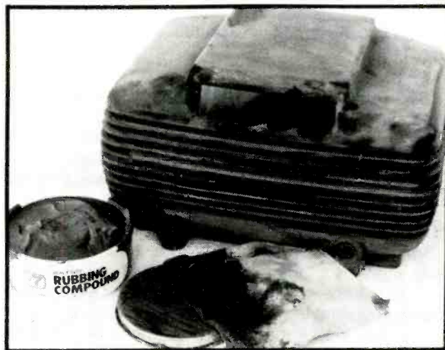
Photo #9. Polishing out scratches with rubbing compound.
