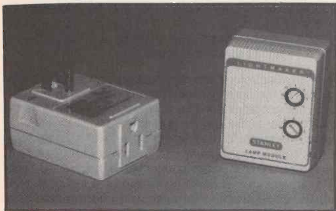
Fig. 1 Stanley Appliance Module (left) and Lamp Module (right). Two rotary switches allow programming of house code and unit code.
