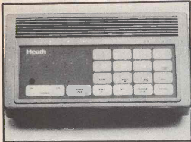
Fig. 11 Heath's innovative House Sitter allows the user to check on the status of his home simply by placing a telephone call. In the event of an emergency, the unit will even call for help.
