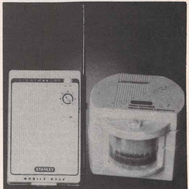
Fig. 8 When the passive infrared sensor picks up movement by an intruder, it beams a radio signal to the base unit at the left, which then rebroadcasts the information over the AC power lines, causing lights to go on or an alarm to sound.
