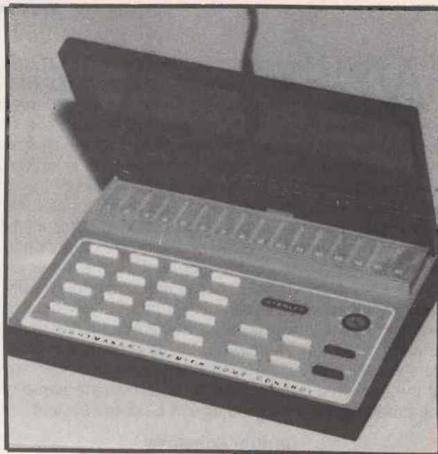
Fig. 2 Stanley Premier Home Control is capable of controlling up to sixteen devices and dimming lamps, too.
