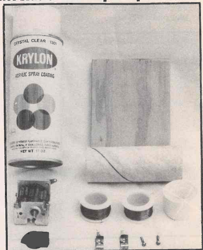
PHOTO #1—Parts required to build the Rejector, including acrylic spray and double-sided mounting tape.
