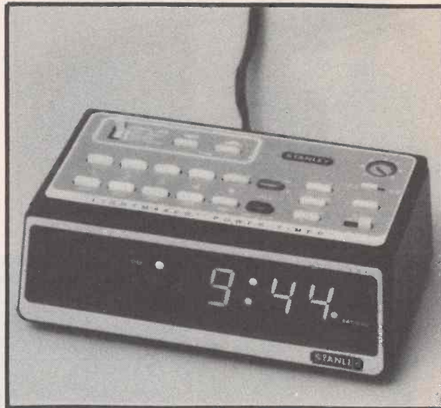
Fig. 4 This Power Timer unit from Stanley can be programmed for on/off control of any X-10 compatible device and also functions as a handy digital clock.
