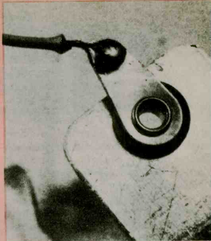
This picture shows a good soldered joint. It has enough solder to hold securely and make a good electrical connection. It has not too much solder, not too little.
