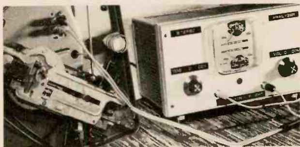
Figure 8. Where to connect the cables from analyzer to the turntable.
