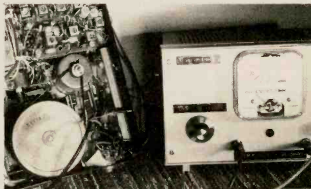
Figure 9. Checking out the amp in a stereo tape player.
