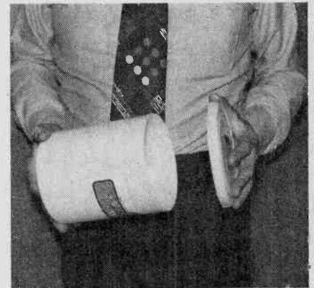
Plastic food container gets cut off near top to secure cover which seals speaker.
