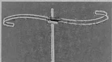
Two different types of omnidirectional antennas. Each one provides a pattern of sensitivity that is as nearly circular as possible. With these units an antenna rotator is unnecessary since nothing is gained by turning them, although the lack of a reception pattern concentrated in one direction means that a lot of sensitivity is lost.
