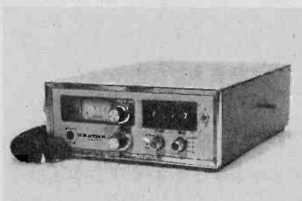
Some of the schools include amateur radio communications equipment kits, such as this Heath HW-2036 VHF FM transceiver.
