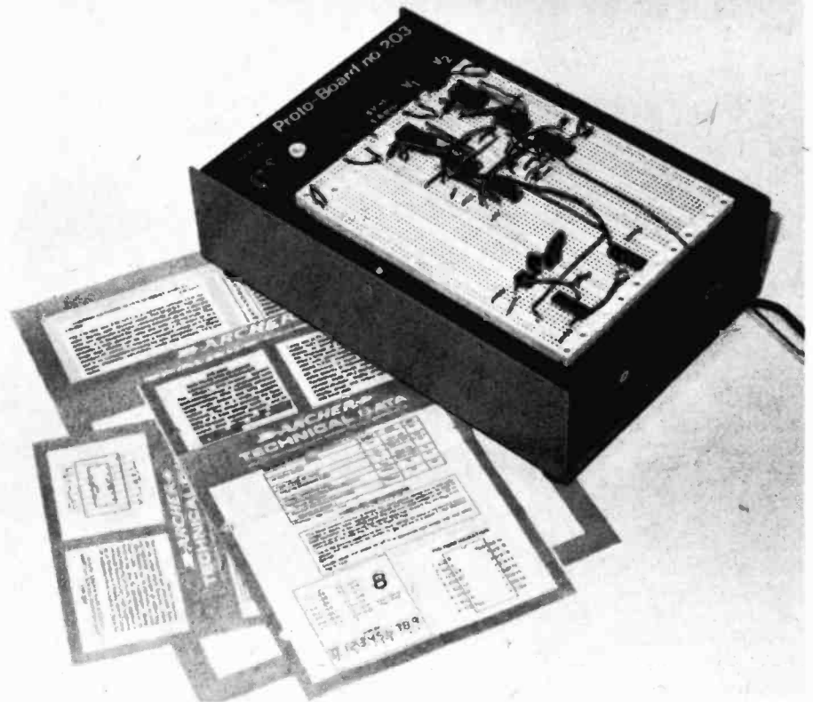
The CSC Proto-Board made experimentation a snap. Connections could be swapped around without muss or fuss. Hang on to the data sheets that come with IC chips, they are an invaluable reference source. Some, like the Radio Shack/Archer ones shown here, have lots of ideas for future experimentation and circuit design modifications.
