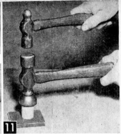
Small world globe makes a good sphere (top to bottom). After paint is removed, hole in bottom half is enlarged with duckbill tin snips to about 13/16 -in. diameter. Pair of hammers and a homemade die put a smooth well-rounded edge on the hole for a press fit on plastic column.
