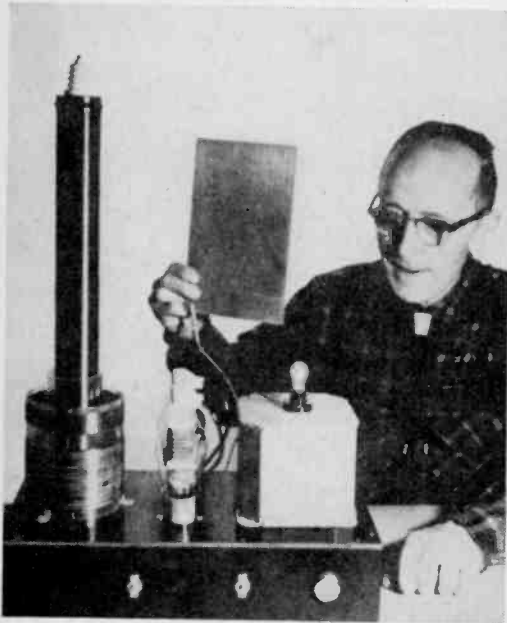
Fig. 6: A sheet of aluminum held in the hand serves as antenna, helps light a small incandescent lamp.
