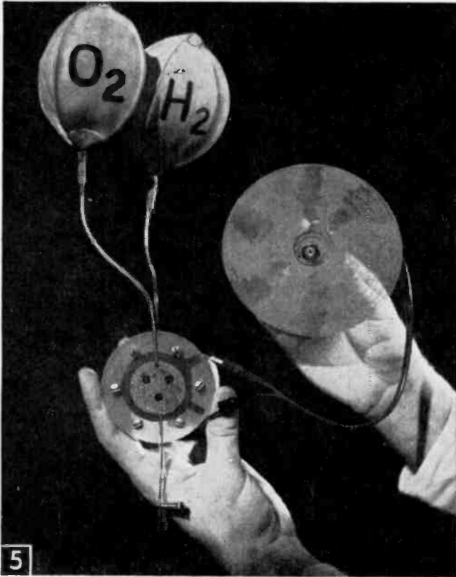
5 Rubber respirator bags filled with purchased hydrogen and oxygen run Aristo-Rev midget motor and 6-in. propeller for several hours.
