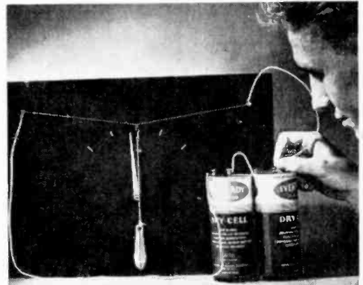
Increase the temperature between the two nails and the pointer will move like an ammeter or temperature indicator in a car.
