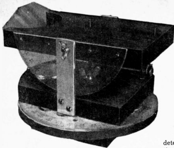
An accurate homemade transit for measuring vertical and horizontal angles.
