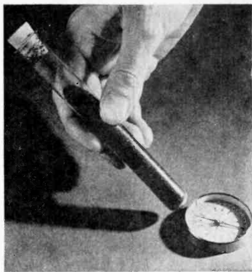
Fig. 3: Magnetized iron filings can also be used to illustrate the molecular theory of magnetism.
