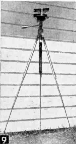
Homemade transit mounted on camera tripod.
