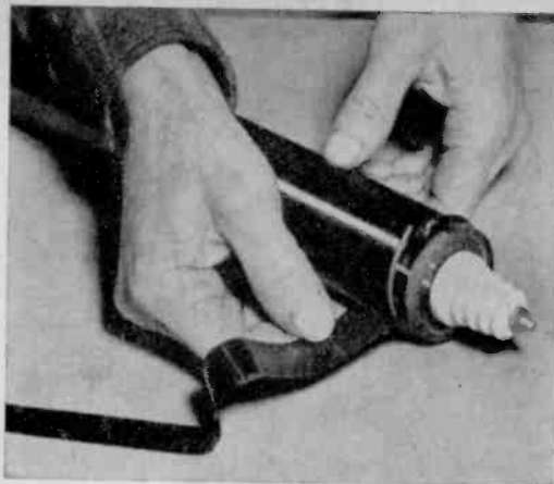
Fig. 14: Put the top disk in place and again, apply tape to finish, as on the bottom and overlap.
