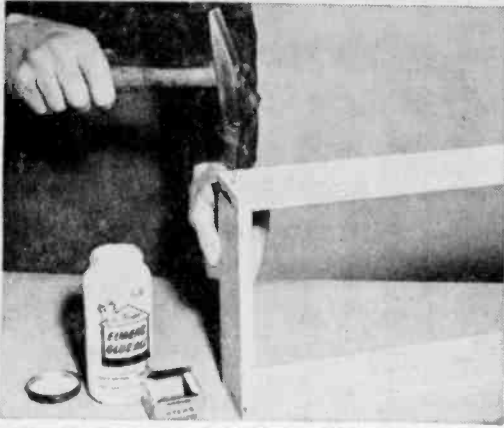
Fig. 21: The base is assembled with wire brads and Casein cement. Follow dimensions given in diagrams.
