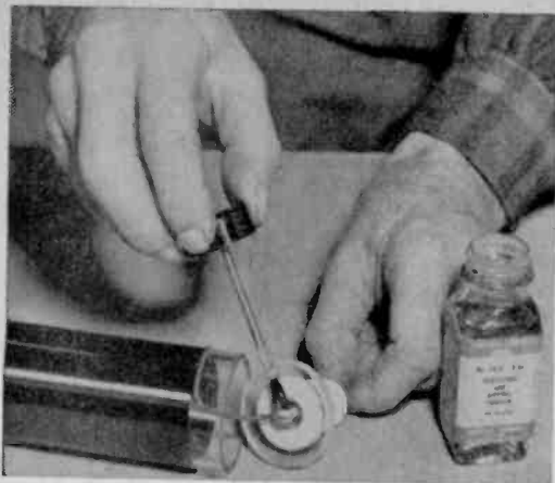
Fig. 13: After mounting the porcelain insulator on the top disk, use corona dope on the screw head.
