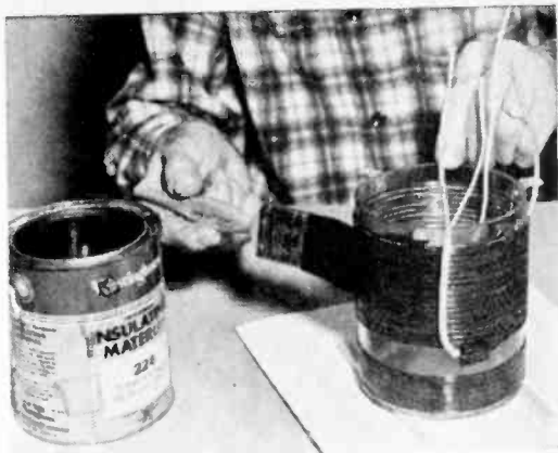
Fig. 18: Apply two coats of insulating material, either by spraying or brushing, as above, let dry.
