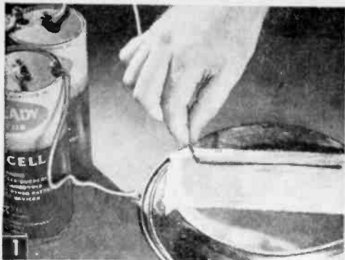
With dry cell batteries, you can draw a line with direct current—and make dots when the current is supplied by a doorbell transformer.
