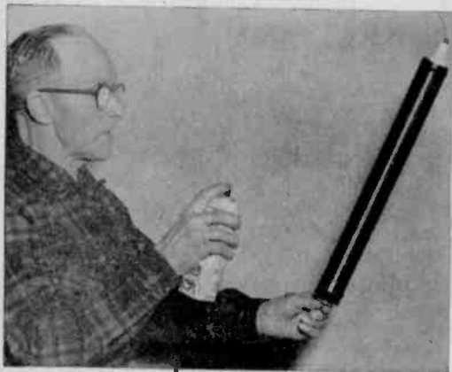
Fig. 15: Carefully apply at least two coats of a good spray-type insulation. Allow each coat to dry.
