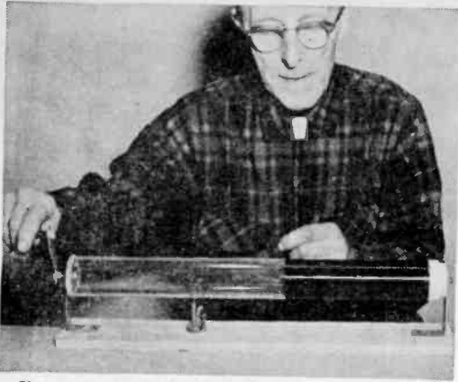
Fig. 9: A simple hand-winding jig can easily be assembled to facilitate winding the larger coil.
