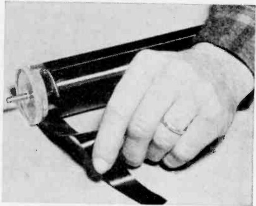
Fig. 12: Finish with a strip of electrical tape, making sure you have sufficient overlap to cover.
