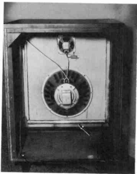
Fig. 605. Humidity problems may necessitate use of a resistive heating unit to protect certain components against excessive moisture. This unit is designed especially for use in closed cabinets. If cabinet is tightly sealed, the manufacturer recommends drilling several small holes to allow ventilation. (Dampp-Chaser, Inc.)
