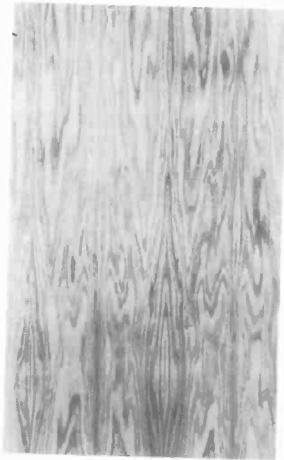
Fig. 1208. A gentle swirl in the graining figure is an identifying feature of plain sliced oak. (Hardwood Plywood Institute.)
