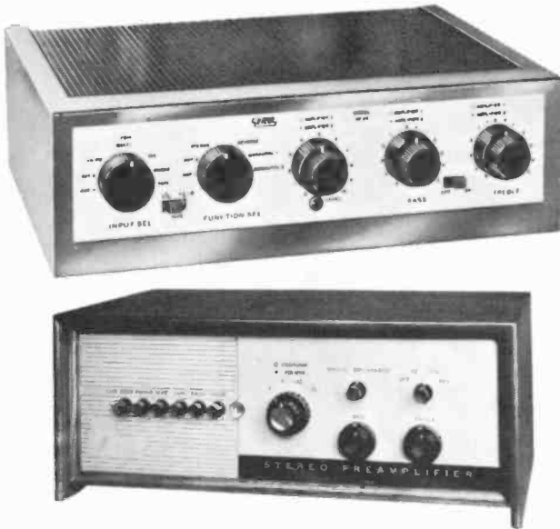
Fig. 411. Preamplifiers must perform many functions in a stereo system. Complex switching systems take some of the brainwork out of operating the rig, but a customer can be frightened by "all those knobs" if he doesn't understand their purpose. (Upper photo: Electronic Instrument Co. Lower photo: Altec Lansing Corp.)
