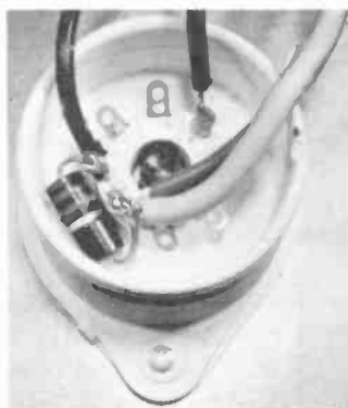
Fig. 908—Broad vertical lines of noise are usually caused by internal corona in high-voltage rectifier. 1,000- or 1,500-ohm resistor wired between tube filament and regulator/picture-tube wires will reduce noise.
