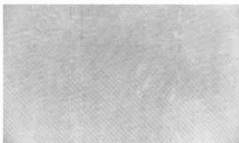
Fig. 623—"Screen-wire" pattern caused by not trapping or filtering out 3.58-MHz signal from demodulator circuitry.
