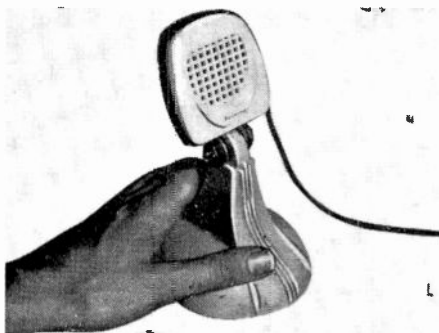
Fig. 410. Base of old fan can be used as support for mike.
