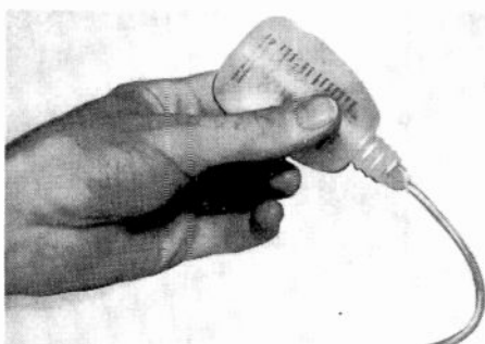
Fig. 411. Plastic bottle with added nozzle gets lubrication into tight spots.
