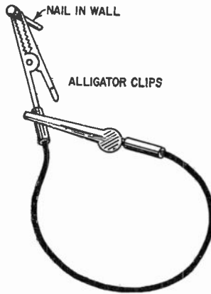
Fig. 503. Simple way of keeping jumpers untangled and ready for use.
