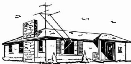
Fig. 213. Some clothesline will help you solve the problem of orienting the TV antenna when you do the job alone.
