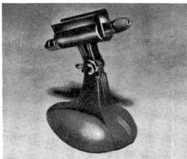
Fig. 547. Paper clamp and old metal base join forces to make handy vise.
